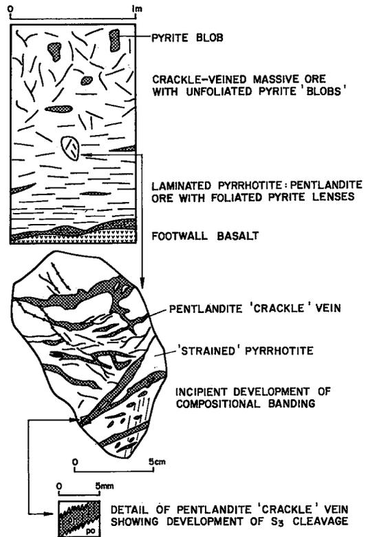
FIG. 3. Sketch of medium-tenor sulfides from the 1050 stope, 50 surface, Juan complex (KNO grid co-ordinates 55139&N, 371703E, +88 m R.L.), showing the progressive development of banded massive sulfides from crackle-veined massive sulfides. Note the flattening of amoeboid pyrite blobs and the overprinted  $S_3$  cleavage.
