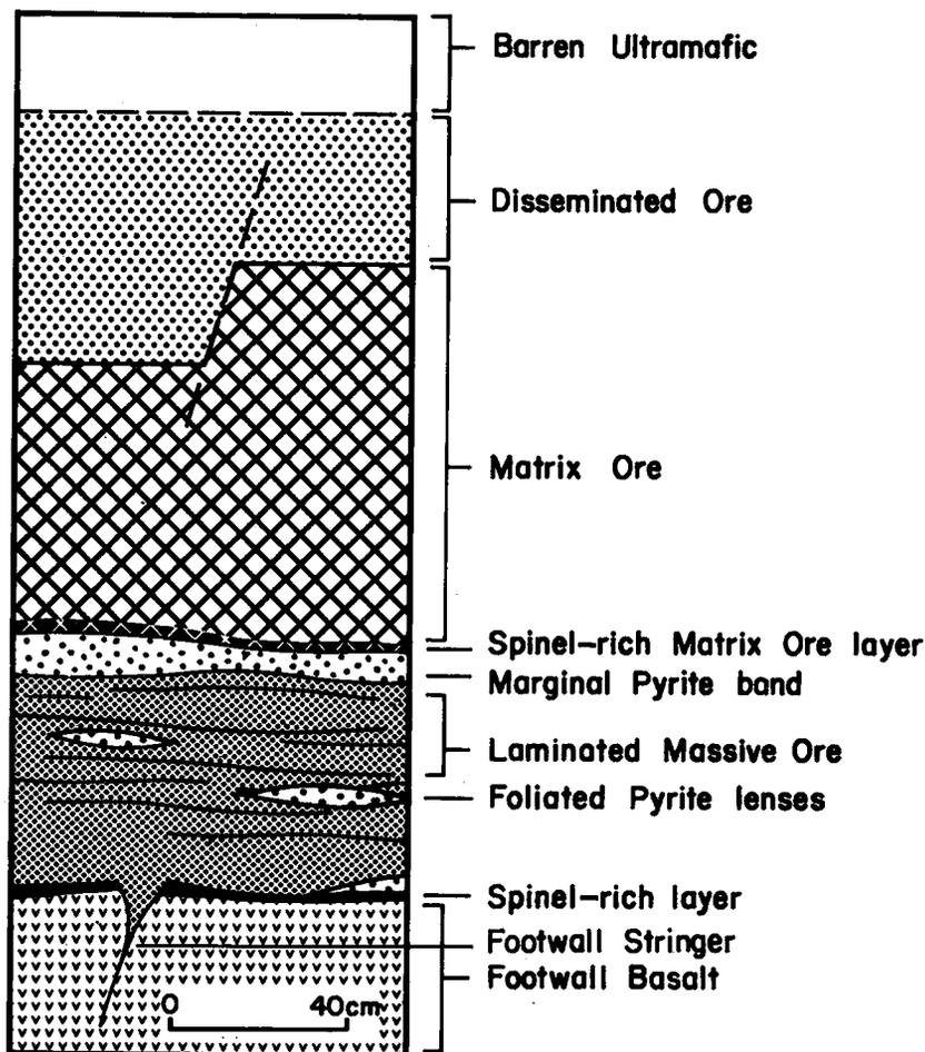
FIG. 1. A schematic sketch of a typical section through the ore zone.
