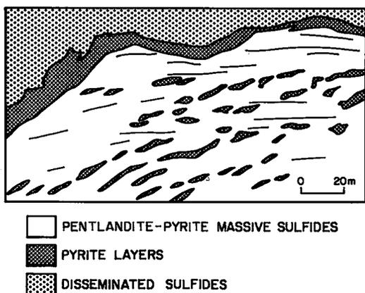
FIG. 7. Sketch of high-tenor massive sulfides from the 234 stope, Banana surface, Juan complex (KNO grid coordinates 550300N, 371595E, +281 R.L.). Foliated but poorly banded massive sulfides contain abundant fine-grained foliated pyrite lenses (type 3) resembling a flaser texture. Note the marginal pyrite band (type 4) at the upper massive-sulfide boundary.
