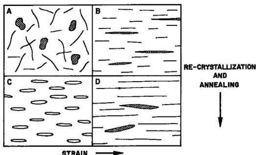
FIG. 6. Textures in massive sulfides as a function of degree of stress and annealing. A. Coarse-grained, crackle-veined massive sulfide containing blobs of fine-grained pyrite. B. Fine-grained, foliated massive sulfides containing flattened foliated fine-grained pyrite lenses. C. Coarse-grained, poorly-banded massive sulfide. D. Coarse-grained, well-banded massive sulfide containing flattened foliated pyrite lenses.
