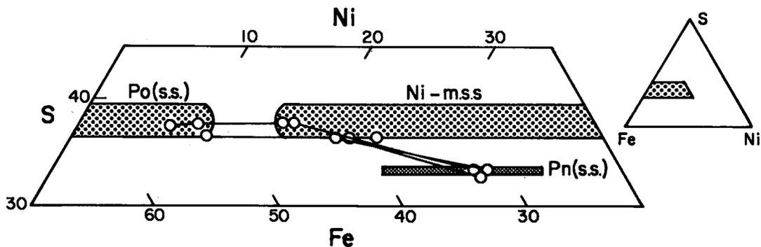
FIG. 9. Portion of the system Fe-Ni-S at 500 to 540°C and one atmosphere, showing our interpreted phase-relationships and the results of McQueen's (1979b) experiments (open circles). Stable assemblages for low- and medium-tenor compositions are Ni-poor *Mss* (Po solid solution + Ni-rich *Mss*), and Ni-rich *Mss* + pentlandite for high-tenor compositions.
