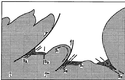
FIG. 5. Sketch cross-section of the D Zone Deeps area, Hunt shoot (cross section no. 84). Note the folding of an  $S_1$  foliation by  $F_2$  recumbent folds and obliteration of  $S_1$  banding in sulfides by  $S_2$  foliation associated with thrusting in pinchouts. Upright  $S_3$  cleavage overprints these fabrics.
