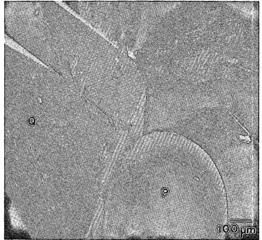
FIG. 2. Scanning electron photomicrograph of pyrobitumen (P) on quartz (Q). Scale in millimeters.
