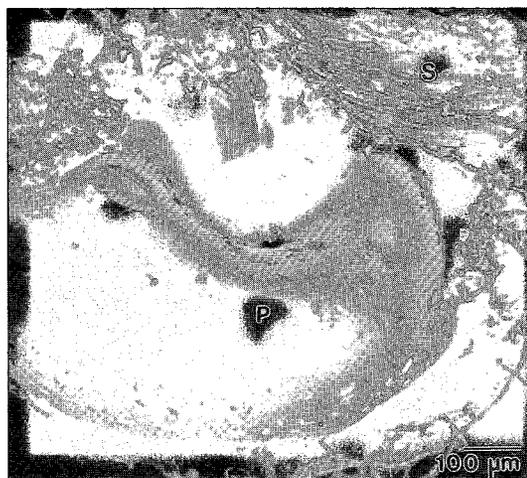
FIG. 5. Scanning electron photomicrograph of pyrobitumen (P) partially encased in sepiolite (S).
