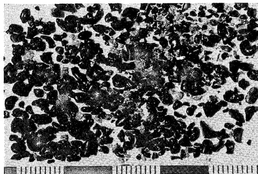
FIG. 7. Blebs of pyrobitumen illustrating round, elongate, twisted and other forms. Scale in millimeters.
