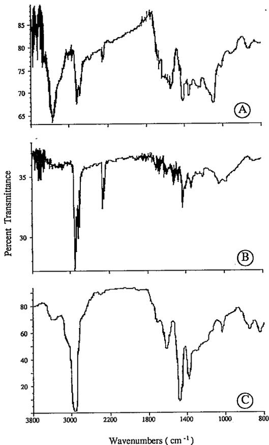
FIG. 8. Infrared absorption spectra: A. pyrobitumen from the Panel mine, B. bitumen from the Ordovician Trenton Formation, and C. standard bitumen (LeDoux & Company, 1986, pers. comm.).
