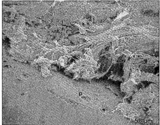
FIG. 12. Scanning electron photomicrograph illustrating vesicles in a bleb of pyrobitumen (P) partially encased by sepiolite (S).
