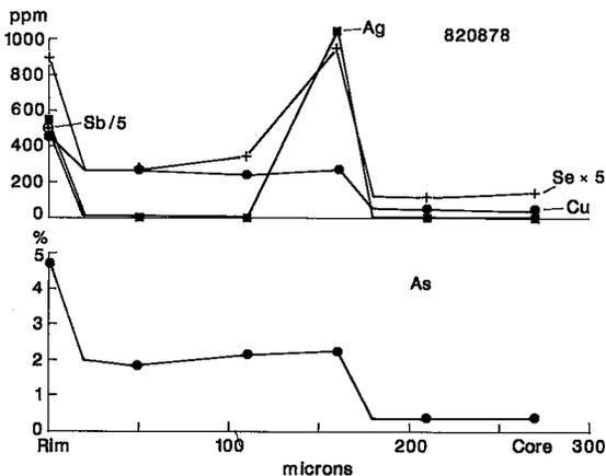
FIG. 5. Concentration of some elements along a point traverse from core to rim, across the pyrite grain shown in Figure 2a.
