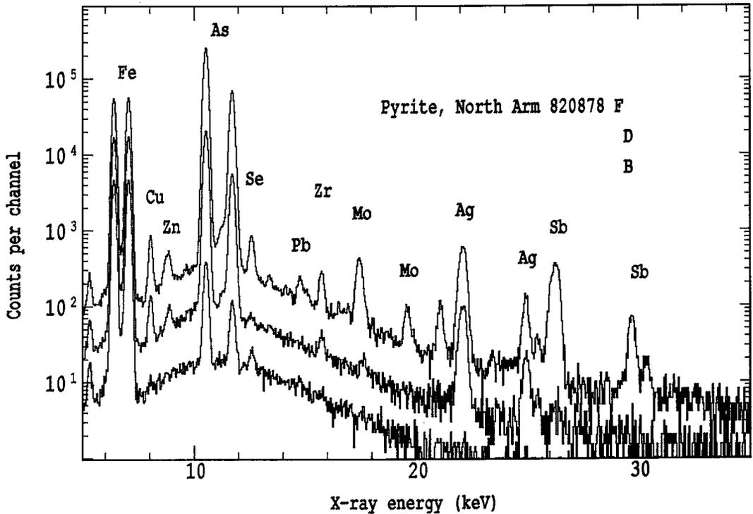
FIG. 3. PIXE spectra of three pyrite grains of varying As content in sample 820878.
