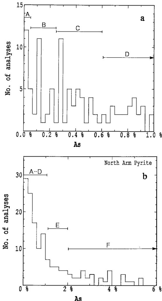
FIG. 4. Histogram showing distribution of As in point analyses collected in this study. Groupings used for summed spectra are indicated by horizontal lines labeled A, B, etc.
