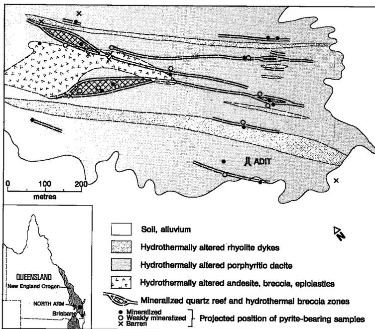
FIG. 1. Location and geology of the North Arm Au-Ag deposit, southeastern Queensland, showing locations of pyrite samples (projected to the surface).
