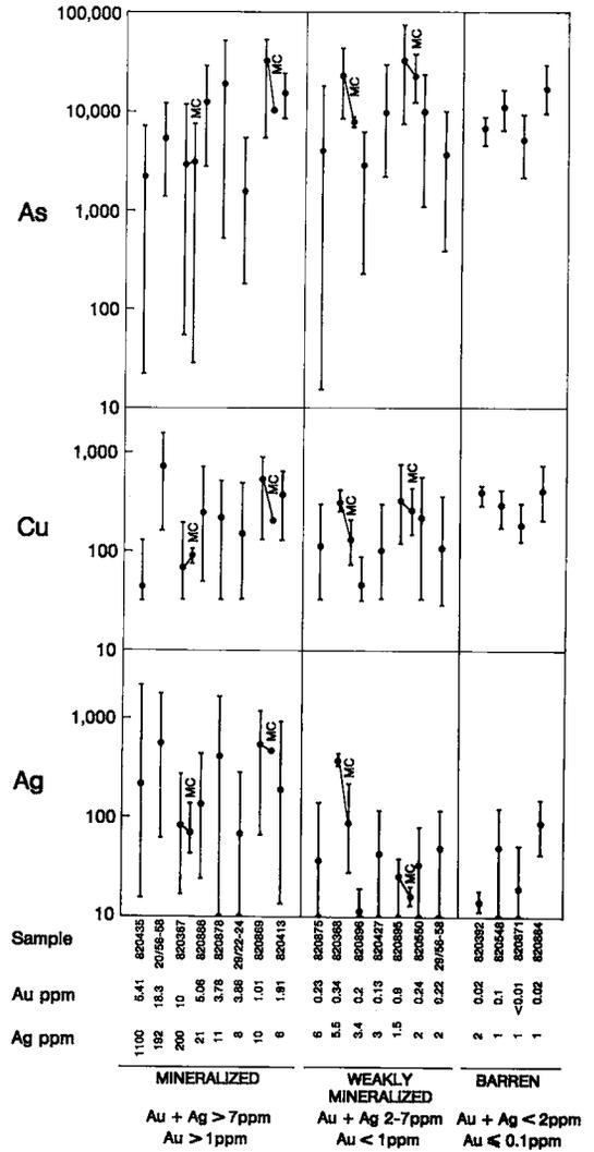
FIG. 11. As, Cu and Ag variations in pyrite and marcasite from the North Arm deposit in relation to bulk sample Au and Ag content. Bars represent ranges of elements detected in individual samples, black dots, the arithmetic means. MC signifies ranges for marcasite; remainder are for pyrite. Tie lines connect means of pyrite and marcasite from each sample. Element contents are in parts per million.
