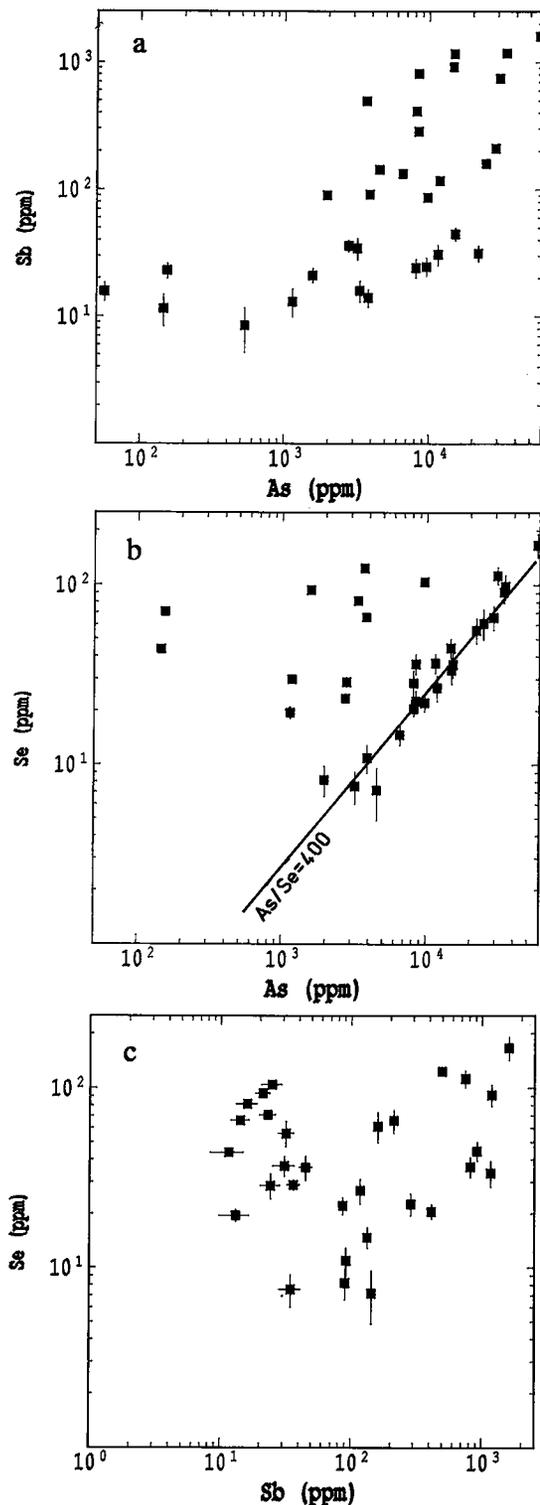
FIG. 7. As-Sb-Se relations in pyrite (summed spectra); data from Table 1.
