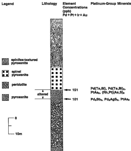
FIG. 2. Schematic section through the Boston Creek Flow showing locations, bulk  $\Sigma(\text{Pd} + \text{Pt} + \text{Ir} + \text{Au})$  values (ppb), and the PGM found in the two mineralized occurrences.
