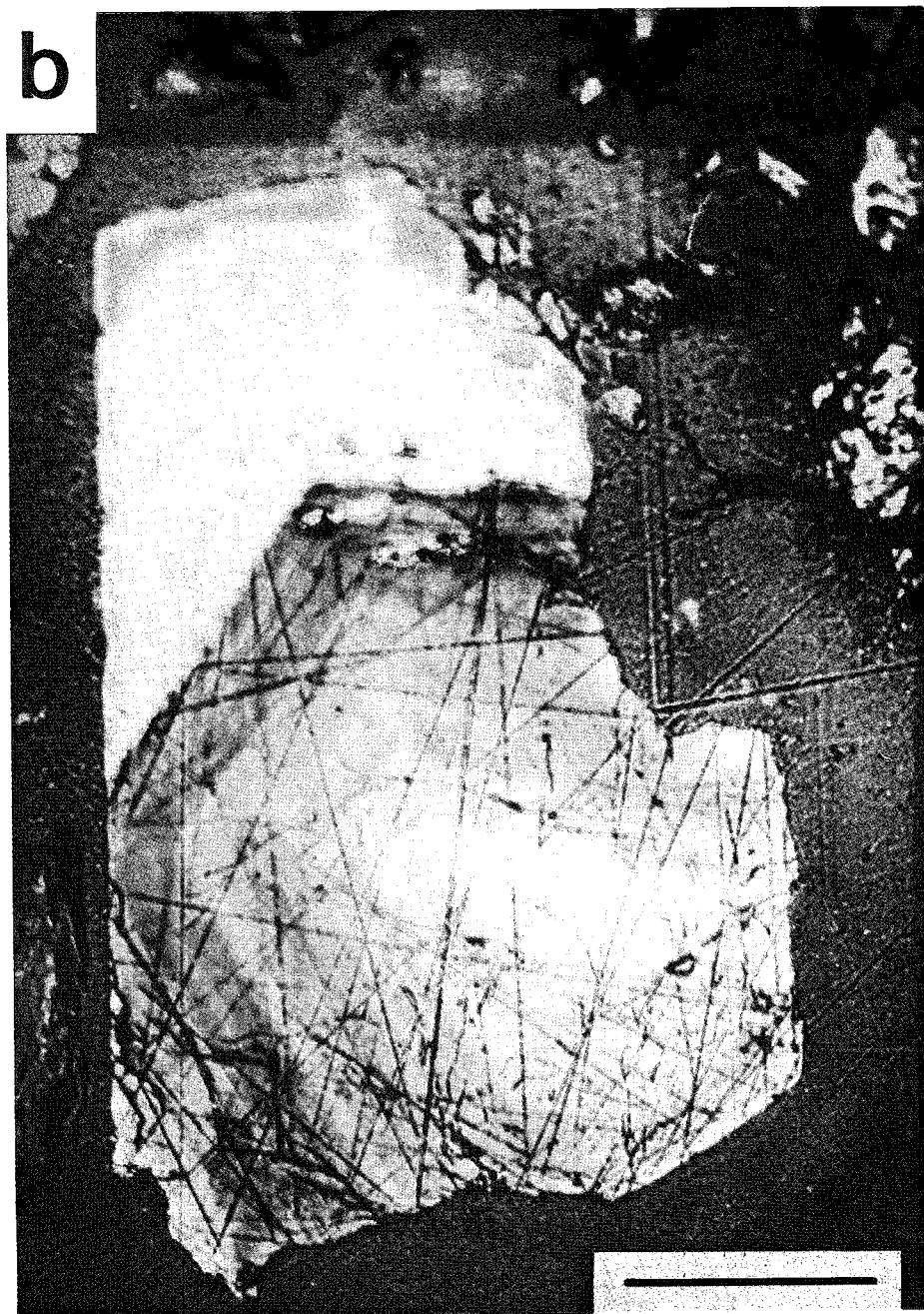
FIG. 3b. Arsenian pyrite grain from sulfidic reef of Fairview mine (sample 17359). Optical micrograph of polished section stained with \text{KMnO}_4 and showing As-rich growth bands (purple, red). Scale bar is 0.1 mm.
