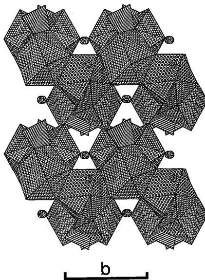
FIG. 4. The dietzeite structure projected onto (001). I atoms are shown as circles shaded with a random dot pattern. The polyhedral shading is as in Figure 2. All I- $\phi$  bonds have been omitted ( $\phi$ : unspecified anionic group).
