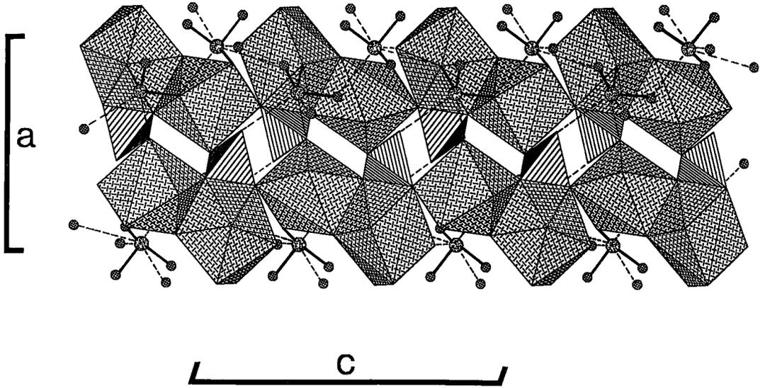
FIG. 5. The dietzeite structure projected onto (010). The polyhedral shading is as in Figure 2. I atoms are given as circles shaded with a random dot pattern, and oxygen atoms are cross-hatched circles. Short I-O bonds are drawn as solid lines, and long I-O bonds, as broken lines ( $\phi$ : unspecified anionic group).
