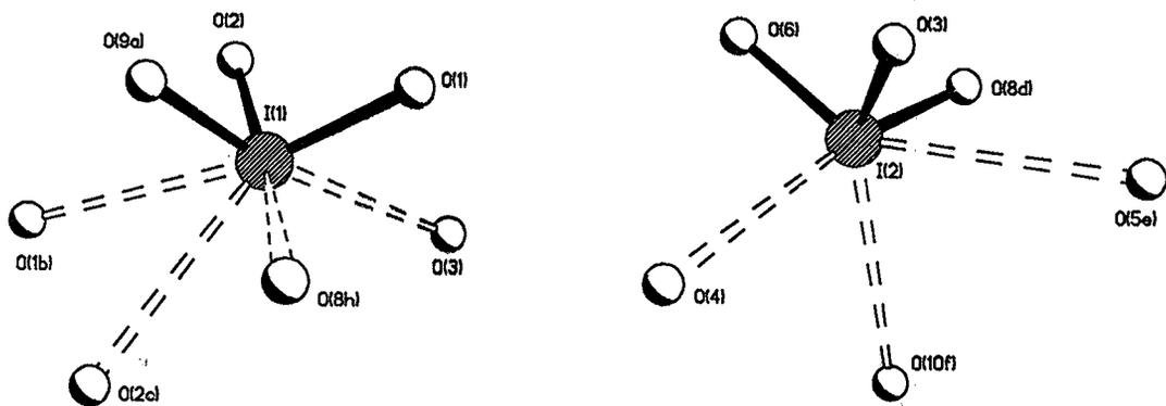
Fig. 1. The I coordination polyhedra observed in dietzeite. Short bonds are given as solid lines, and long bonds are given as broken lines.
