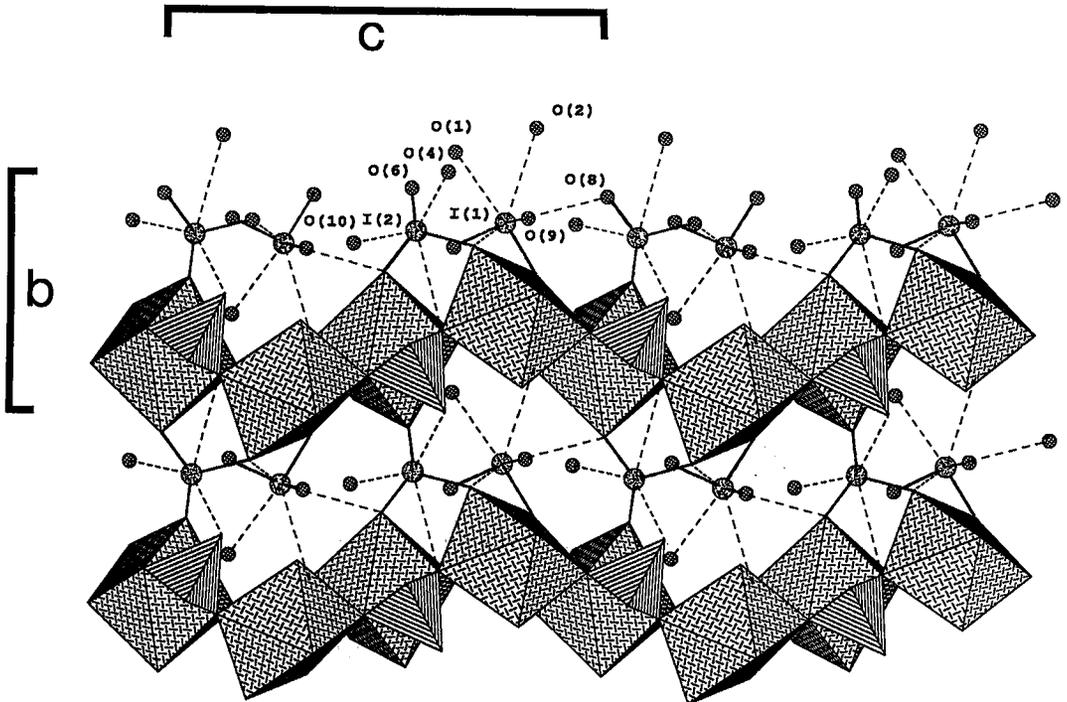
FIG. 6. The dietzeite structure projected onto (100). Legend as in Figure 5.
