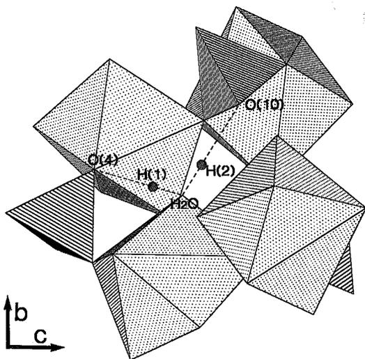
FIG. 2. Proposed scheme of hydrogen bonding in dietzeite. The O-H and H...O bonds are shown as broken lines. Ca polyhedra are shaded with a regular dot pattern, and Cr tetrahedra, with parallel lines.
