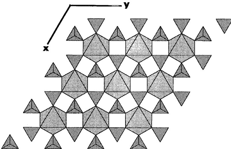
FIG. 3. A z-axis projection of the  $[\text{Ca}(\text{PO}_4)_2]$  structural layer, which is composed of  $[\text{CaO}_6]^{4-}$  polyhedral trigonal antiprisms connecting  $[\text{PO}_4]^{3-}$  tetrahedra.
