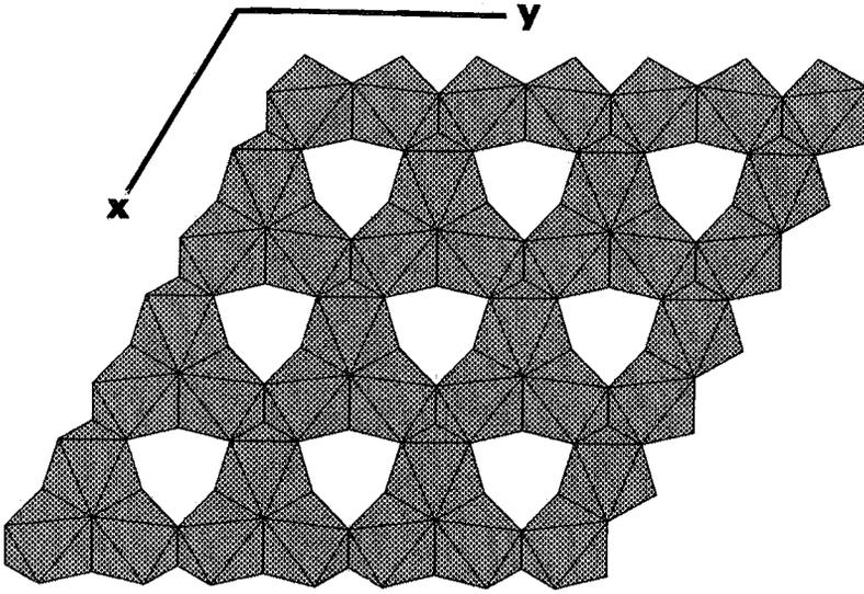
FIG. 2. A z-axis projection of the structure of harrisonite showing the corundum-type  $[\text{FeO}_6]^{10-}$  layer.
