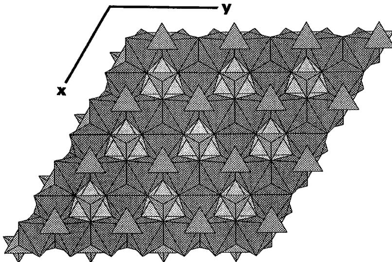
FIG. 4. A z-axis projection of the structure of harrisonite. The  $[\text{FeO}_6]^{10-}$  layer has  $[\text{SiO}_4]^{4-}$  tetrahedra capping the top of the layer holes and  $[\text{CaO}_6]^{10-}$  polyhedra underlying the holes.
