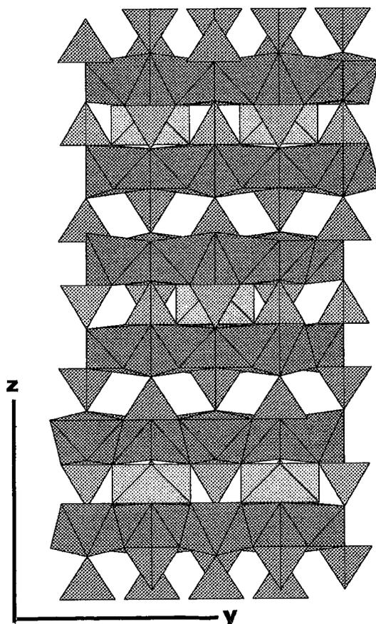
Fig. 1. A (100) projection of the layered structure of harrisonite, with dark-shaded  $[\text{SiO}_4]^{4-}$  tetrahedra, lighter-shaded  $[\text{PO}_4]^{3-}$  tetrahedra, light-stippled  $[\text{CaO}_6]^{10-}$  polyhedra, and dark-stippled  $[\text{FeO}_6]^{10-}$  polyhedra.
