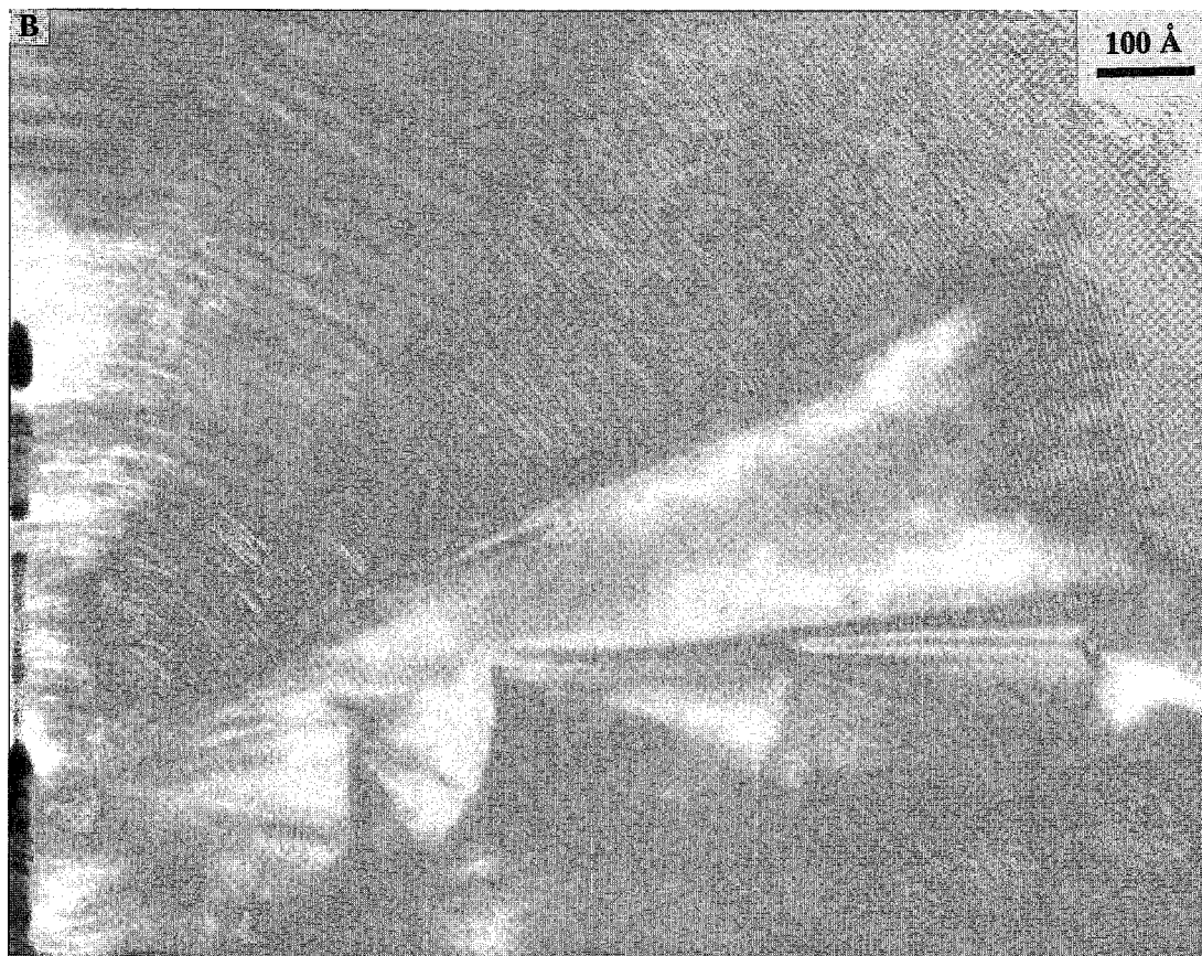
FIG. 9. High-resolution TEM image of a polygonal serpentine fiber, specimen 18501 (see Cressey & Zussman 1976). (A) The whole fiber section and (B) enlarged detail from part of (A), showing flat layers passing coherently across sector boundaries and continuing laterally into curved sheets. Note also the degree of disorder between layers in curved sheets near the fiber center.
