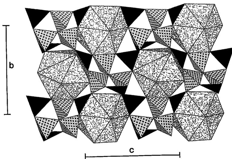
FIG. 2. The heteropolyhedral sheets in tunellite projected onto (100). Borate tetrahedra are shaded with crosses, borate triangles are given as solid triangles, and  $Sr\phi_{10}$  polyhedra are shaded with a random-dot pattern.
