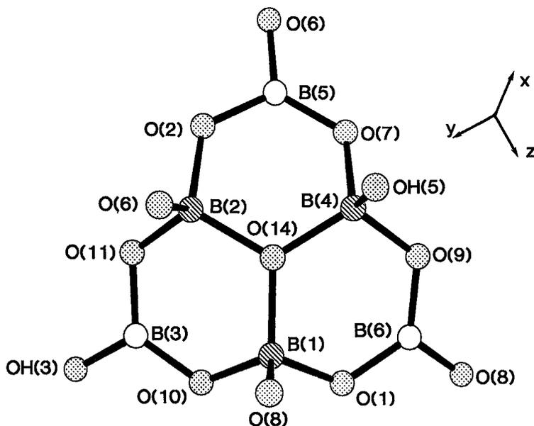
FIG. 1. The hexaborate fundamental building block in tunellite;  $^{[3]}B$  atoms are unshaded circles,  $^{[4]}B$  atoms are line-shaded circles, and anions are dot-shaded circles.
