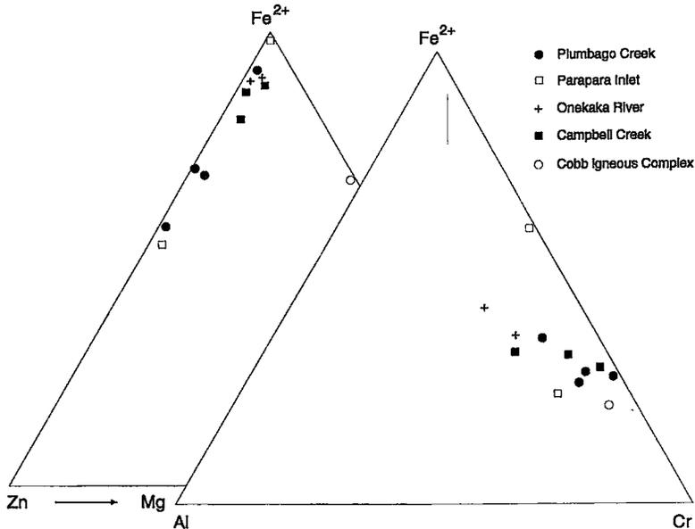
FIG. 10. Composition of zincian chromite from Plumbago Creek, Parapara Inlet, Onekaka River, and Campbell Creek, together with that of high-Cr chromite from the Cobb Ultramafic Complex.
