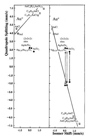
FIG. 1. Quadrupole splitting (QS) – isomer shift (IS) correlation for Au<sup>+</sup> compounds. Left: the correlation proposed by Wagner et al. (1994). The solid line is the assumed correlation, and full dots show the hyperfine parameters of <sup>197</sup>Au in (2 + 2 + 2) sites. Right: The solid line shows the proposed QS–IS correlation (Stanek 1982), with full dots as at left, but with two possible assignment of the sign of V<sub>--</sub>, here the sign of QS.
