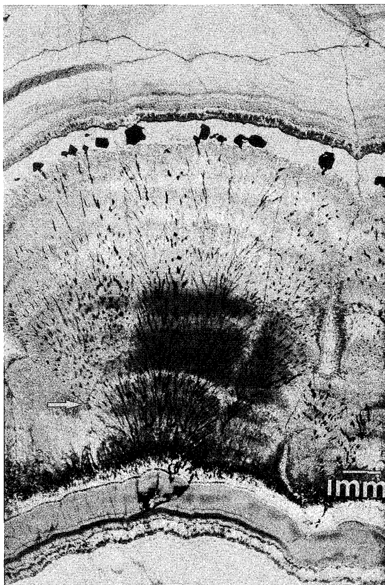
FIG. 1. Plane-polarized-light photomicrograph of part of a thin section showing sphalerite banding in a sample from the Pine Point deposit. The banding varies from clear, to pale white, to brown, to deep red-orange in color. The concentric bands form coalescent arcuate arrays that emanate from centers of growth. In three dimensions, these form the characteristic hummocky, so-called botryoidal textures. Note that some bands toward the top of the image do not correlate over the entire section. Black blebs and filigrees within the sphalerite bands are elements of what are interpreted to be a branching crystals of galena that radiate from the middle of the thin section. Although it appears discontinuous, in three dimensions, all parts are presumably connected. The arrow demarcates a point common to that of the more detailed Figure 3.
