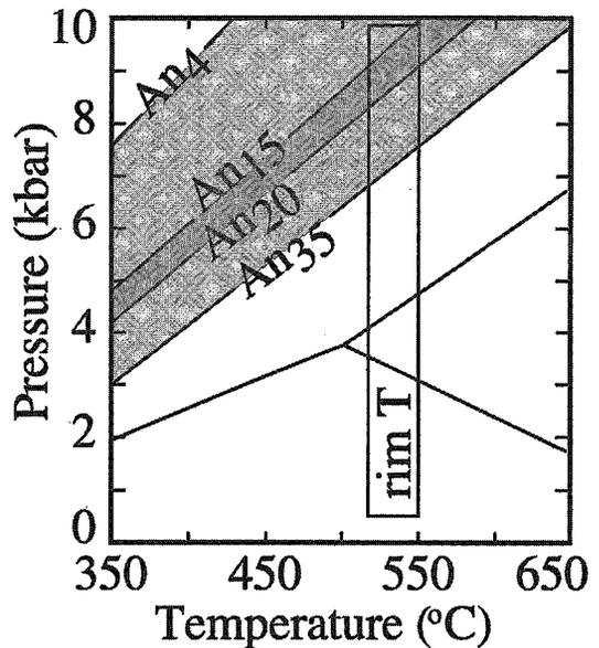
FIG. 10. Thermobarometric estimates for sample EM1B using garnet rim and matrix micas with various plagioclase compositions. The long box outlines barometric estimates possible using all plagioclase rim compositions ( $An_{4-35}$ ). The dark grey band outlines estimates using petrologically reasonable plagioclase compositions,  $An_{15-20}$ .
