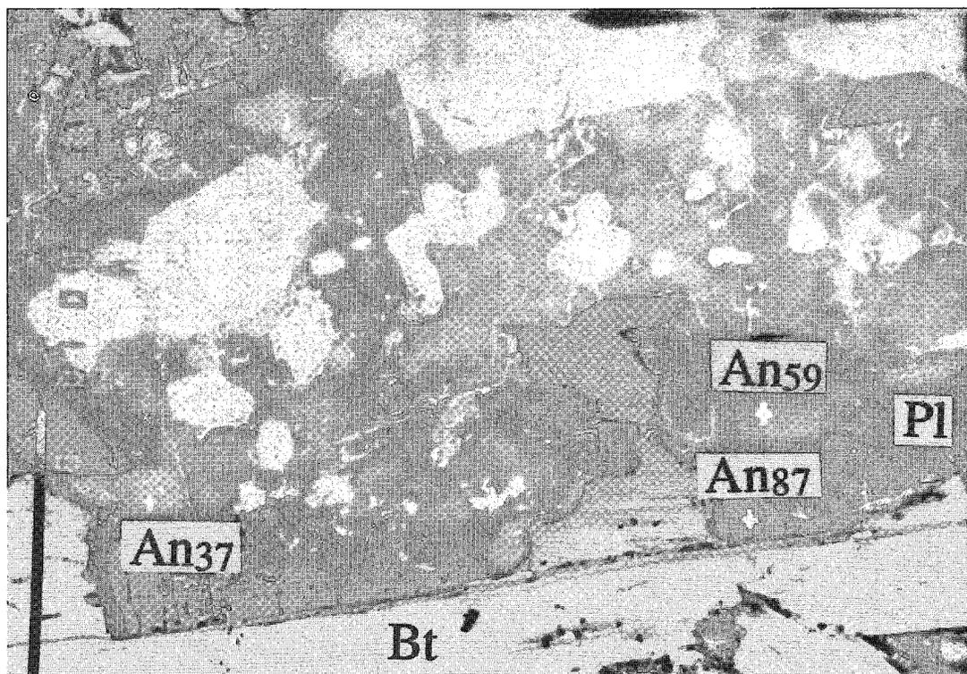
FIG. 7. Patchy zoning in plagioclase. Back-scattered electron image of plagioclase in sample TM732 with compositions as labeled. The zoning pattern follows the shapes of biotite (white), quartz (black), and muscovite (grey mica in upper, left corner).  $An_{37}$  plagioclase is the youngest, as determined by rimming relations. Base of photo is 380  $\mu\text{m}$ .
