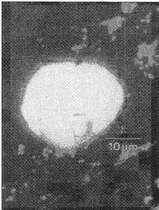
FIG. 1B. Photomicrograph of subspherical grain of cobaltite–gersdorffite<sub>ss</sub>.
