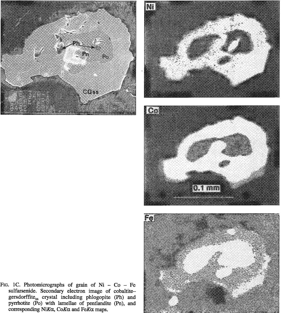
FIG. 1C. Photomicrographs of grain of Ni - Co - Fe sulfarsenide. Secondary electron image of cobaltite-gersdorffite<sub>ss</sub> crystal including phlogopite (Ph) and pyrrhotite (Po) with lamellae of pentlandite (Pn), and corresponding NiK $\alpha$ , CoK $\alpha$  and FeK $\alpha$  maps.
