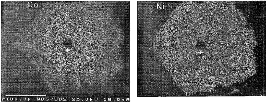
FIG. 1D. Photomicrographs of grain of Ni – Co – Fe sulfarsenide. NiK $\alpha$  and CoK $\alpha$  maps of a euhedral grain of cobaltite–gersdorffite<sub>ss</sub> showing a normal, discontinuous zonation. Scale bar: 100  $\mu$ m.
