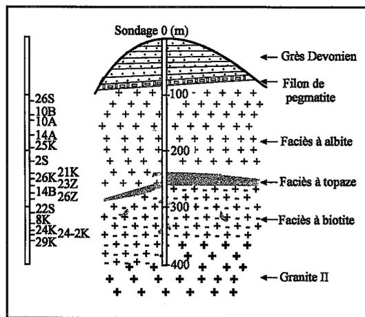
FIG. 1. Cross-section of Granite II at Suzhou, made as a result of observations made on surface exposures and from the drill core. To the left is the position of samples used in this project.
