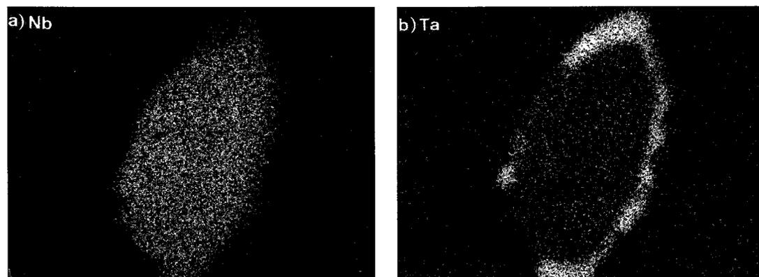
FIG. 3. Images showing the distribution of Nb ( $L\alpha$  radiation, a) and Ta ( $M\alpha$  radiation, b) in a zoned crystal of columbite, and revealing a pattern of Ta enrichment toward the margin. The width of the crystal is roughly 20  $\mu\text{m}$ .
