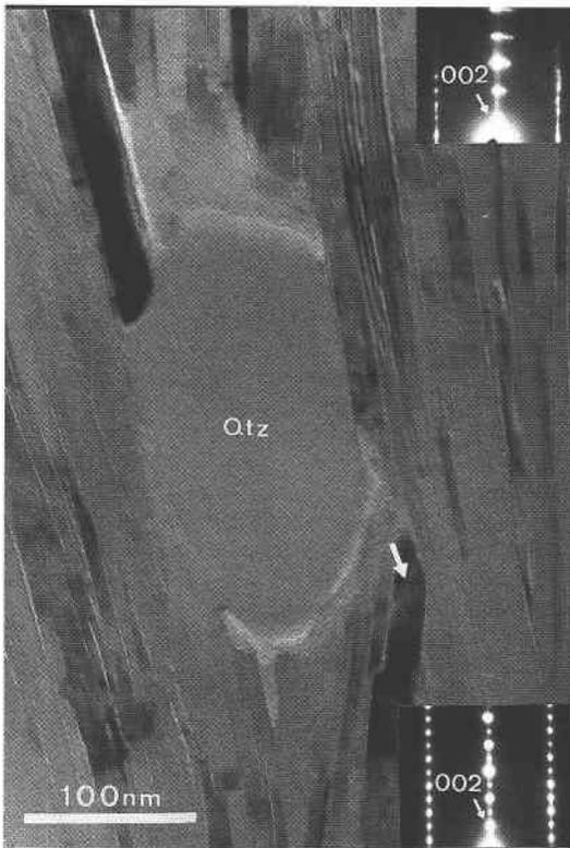
FIG. 3. Lattice-fringe image of thin crystallites of illite in the ion-milled diagenetic (near anchizonal) mudstone SW2. The upper inset SAED pattern shows a  $2M$  polytype of illite of authigenic origin, with a poor degree of ordering in non- $00l$  reflections. The lower inset SAED pattern pertains to a grain of the well-ordered  $2M$  polytype of illite, of possible detrital origin, the position of which is marked by an arrow.
