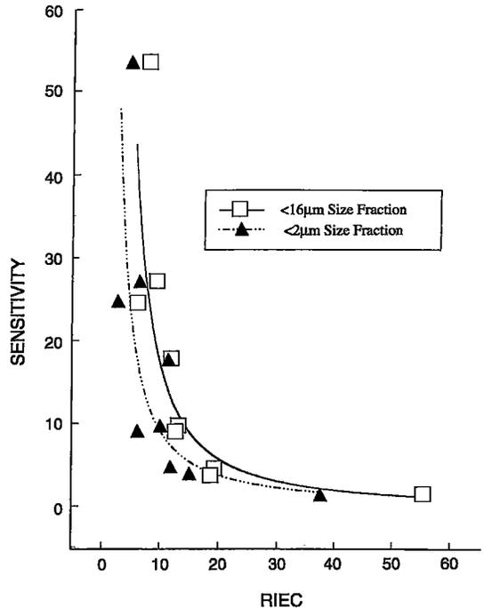
FIG. 5. Sensitivity versus RIEC (Relative Importance of Expandable Clay) index for <16 μm and <2 μm size fractions.
