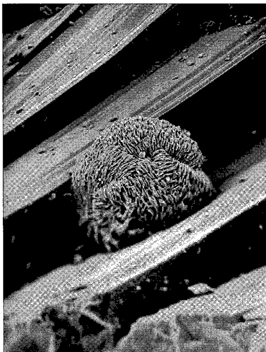
FIG. 4. Spherulite of juonniite on crystals of kovdorskite. Scanning electron micrograph. Width of field of view: 400 \mu\text{m} .
