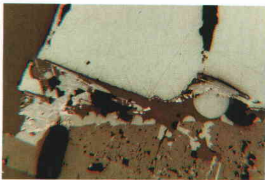
FIG. 2. Reflected-light photomicrograph of realgar (lighter gray phase at top) with intergrown duranusite (thin white lamellae) and sphalerite (intermediate gray phase in spherical masses) and with rhodochrosite (darker gray phase at the bottom). The width of the field of view is approximately 0.6 mm.
