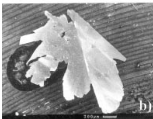
FIG. 3. Morphology of wittite crystals (Se content ranging from \sim 8 to \sim 14 wt%. Variation of color is due to the Se contents; the highest Se contents are in the darkest portions. a) Leaves, scale bar: 100 \mu m, b) elongate tabular crystals, scale bar: 300 \mu m.
