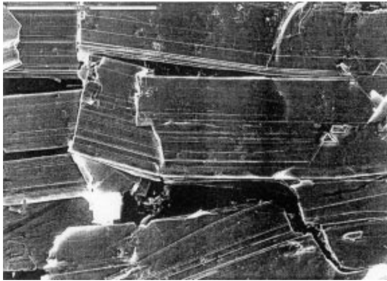
FIG. 4. Striated elongate crystals of wittite ( \text{Se} \approx 10 \text{ wt}\% ) with small crystals of galena on the surface. CamScan 4DV scanning electron microscope. Scale bar: 100 \mu\text{m} .
