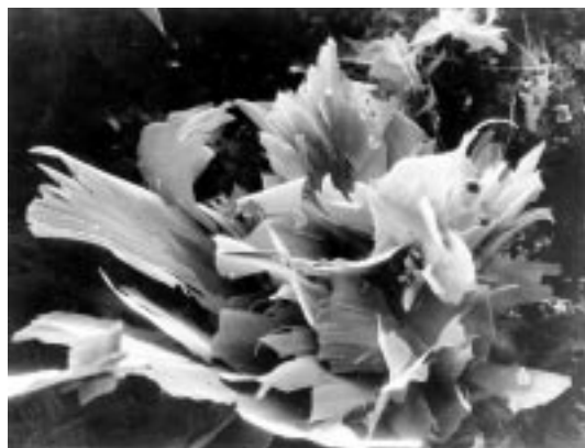
FIG. 2. Aggregate of cannizzarite leaves (Se \approx 2.3 wt%). CamScan 4DV scanning electron microscope. Scale bar: 100 \mu m.
