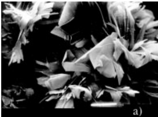
FIG. 5. Relation between cannizzarite ( \text{Se} \approx 3 \text{ wt}\% ) and bismuthinite. a) Idiomorphic prismatic bismuthinite crystals (1) among the cannizzarite leaves, scale bar: 100 \mu\text{m} , b) clusters of cannizzarite minerals on a large crystal of bismuthinite, scale bar: 50 \mu\text{m} . CamScan 4DV scanning electron microscope.
