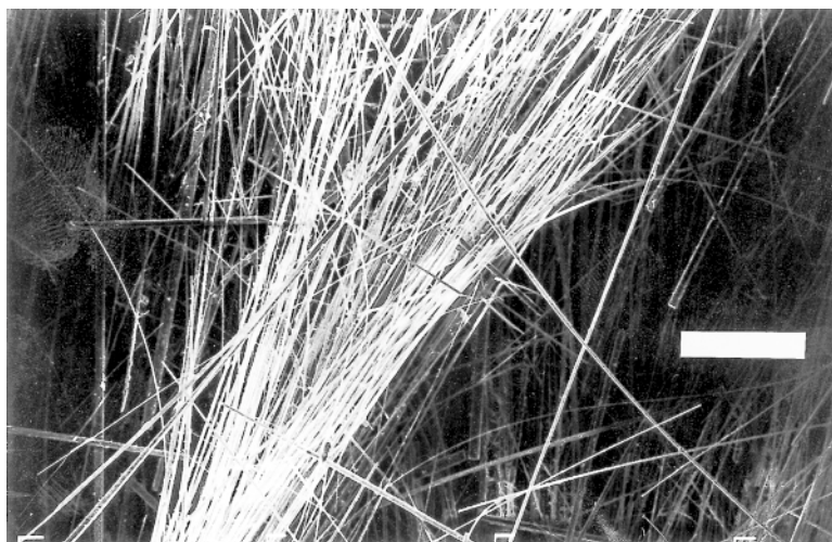
FIG. 1. SEM image of fibrous crystals of ferrian winchite. The scale bar represents 200\text{ }\mu\text{m} .
