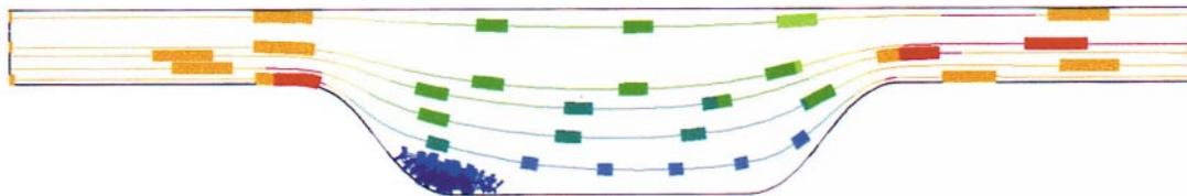
FIG. 6. This is the same configuration as in Figures 4 and 5, but the flow is 10 times more intense than in Figure 5 and 100 times more intense than in Figure 4. In this case, the flow hurdles the hollow, and there is little circulation in it, and therefore little gathering of sulfides. This scenario immediately implies that there are optimum conditions with respect to the Reynolds number for the formation of massive sulfides in embayments.
