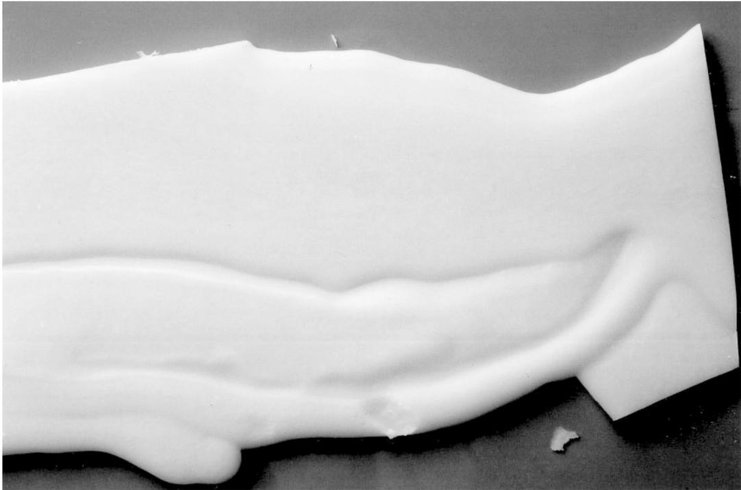
FIG. 8. A similar channel formed from flowing wax. The wax, however, never penetrated the substrate, hence the channel was formed by levee construction and not by thermal erosion.
