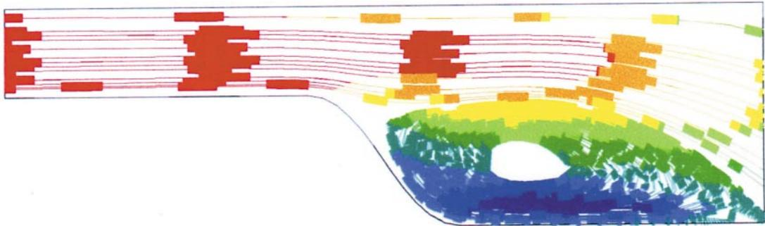
FIG. 2. This is the same configuration as Figure 1, except that the Reynolds number has been increased by a factor of 10 (which can be done by increasing the velocity by 10). Note that the mixing process has become much more powerful in the back eddy, hence the potential deposit would be more massive. Note also that little mixing occurs in the eye of the eddy, which would thus be expected to be more barren of sulfides.
