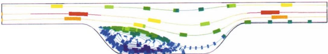
FIG. 4. This figure represents a low Reynolds number (450) flow over a hollow. A small back eddy develops against the upstream wall of the hollow and would be the anticipated zone of deposition of sulfides.
