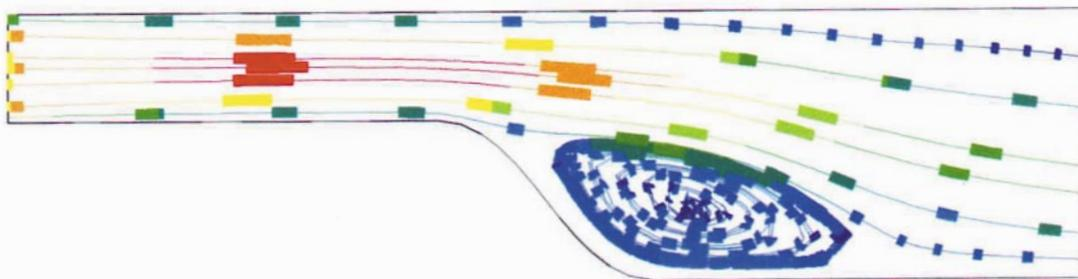
FIG. 1. Particle traces, *i.e.*, the paths that some particles would take in the flow, are depicted here. The views shown for all figures are side views, and the flow is from left to right for all cases given here. In this case, a Reynolds number of 450 typifies the flow. Note the back eddy, which has developed under the ledge or embayment. This eddy will assure mixing of sulfides and melt, to scavenge Ni from the melt.
