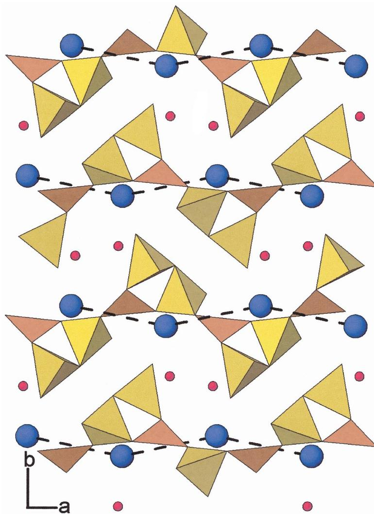
FIG. 5. The structure of colemanite, where the borate chains are parallel to the chains of calcium polyhedra. The  $B\phi_4$  are yellow, and the  $B\phi_3$  units are orange; the Ca-polyhedra are shown as blue circles for simplicity, and the direction of bonding is given by a dashed line.
