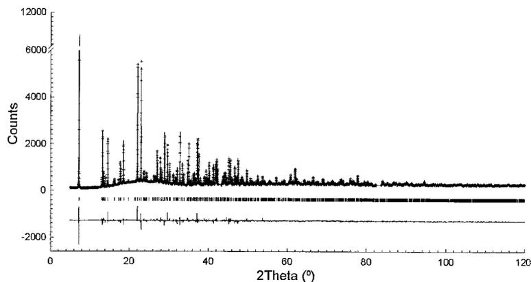
FIG. 1. Powder-diffraction trace for priceite (combined plot of the three histograms). The observed pattern is denoted by +, and the calculated pattern is superimposed. Below that profile are the positions of the Bragg diffraction maxima, and the difference pattern.
