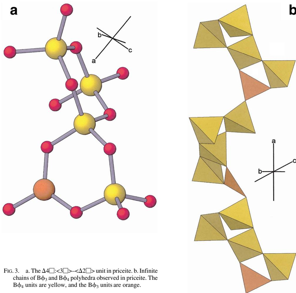
FIG. 3. a. The  $\Delta 4 \square : \langle 3 \square \rangle - \langle \Delta 2 \square \rangle$  unit in priceite. b. Infinite chains of  $B\phi_3$  and  $B\phi_4$  polyhedra observed in priceite. The  $B\phi_4$  units are yellow, and the  $B\phi_3$  units are orange.
