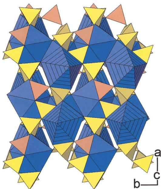
FIG. 2. The structure of priceite.  $B\phi_3$  and  $B\phi_4$  polyhedra are shown in orange and yellow, respectively.  $Ca\phi_8$  polyhedra are blue, with the polyhedra that lie above and below (001) highlighted with hatching.
