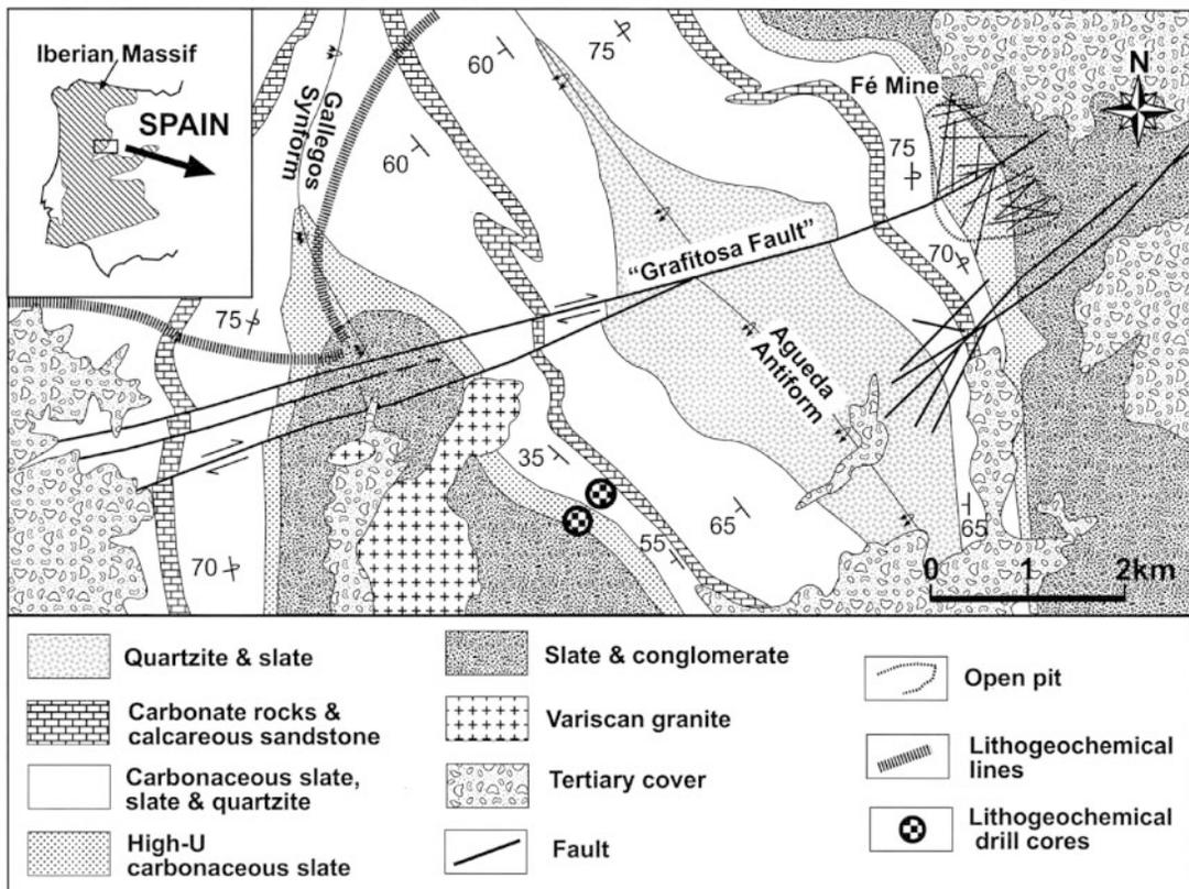
Fig. 1. Regional geological map of the Fé mine area showing the most important stratigraphic and structural features. High-U carbonaceous slates have a U content of >10 ppm.
