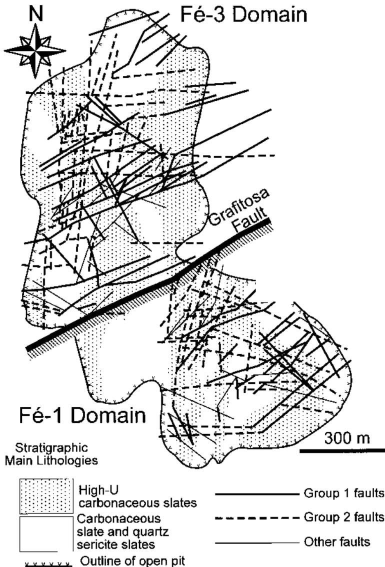
FIG. 2. Geological sketch of the Fé orebody. The two orebodies, Fé 1 and Fé 3, are divided by the Grafitosa fault. The faults affecting both orebodies are distributed in two main groups of conjugate faults, 1 and 2. Note the close relationship between uranium-mineralized faults and stratigraphic levels anomalously enriched in uranium.
