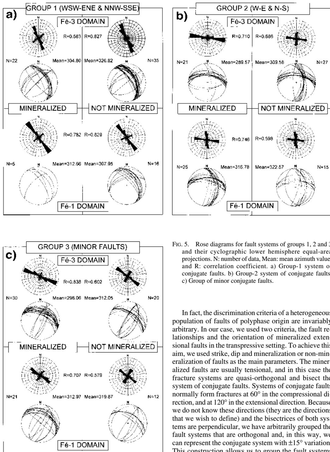
Fig. 5. Rose diagrams for fault systems of groups 1, 2 and 3 and their cyclographic lower hemisphere equal-area projections. N: number of data, Mean: mean azimuth value, and R: correlation coefficient. a) Group-1 system of conjugate faults. b) Group-2 system of conjugate faults. c) Group of minor conjugate faults.
