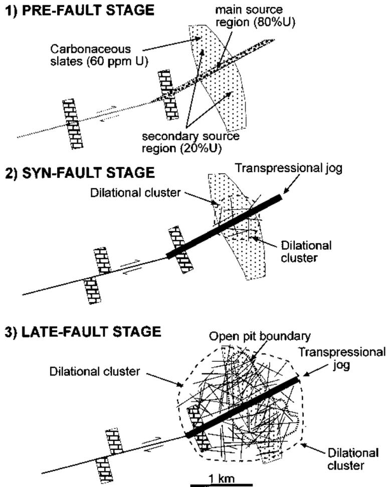
FIG. 8. Genetic model proposed for the deposition of the uranium mineralization in the Fé orebody.
