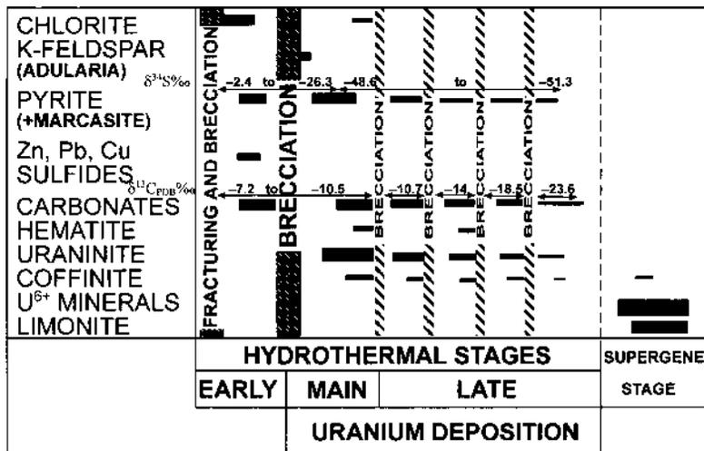
FIG. 4. Paragenetic sequence of mineral deposition (modified after Arribas 1985). Values of  $\delta^{13}\text{C}$  and  $\delta^{34}\text{S}$  have been placed in the relative sequence of mineral deposition.
