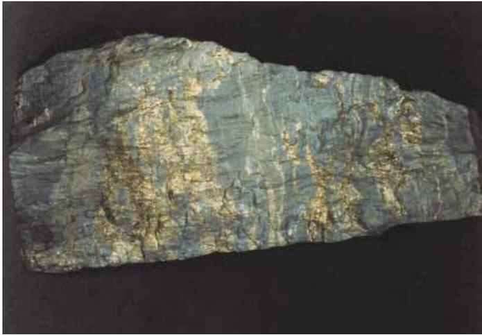
FIG. 9. The MH ore type, Graça orebody. Centimeter-size concentrations of almost pure tetrahedrite-tennantite (bluish grey) are intercalated in banded ores rich in sphalerite (dark grey) + chalcopyrite. Length of the sample: 35 cm.
