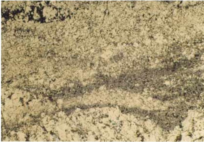
FIG. 16. ME ore type, Corvo orebody. The ore is mostly formed by bands of fine-grained sphalerite in a matrix of porous pyrite that in some places carry small grains of galena (at bottom of the figure). Scale: 20 mm = 720  $\mu\text{m}$ .
