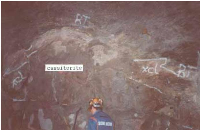
FIG. 19. MT ore type, Corvo orebody. A large meter-sized lens of massive cassiterite located at the top of a lens of massive MC cupriferous ore. At the top of the MT lens, the chloritic schist (xcl) and the tin ore (RT) both form the *rubané* unit.
