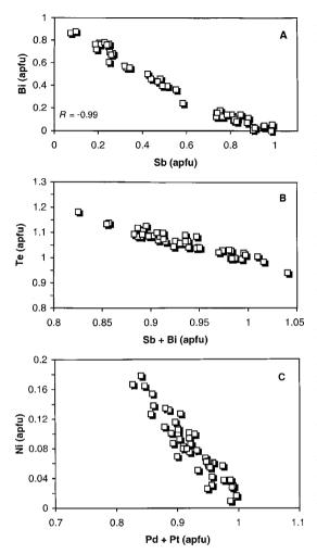
FIG. 8. Concentration of Bi versus Sb (A), Te versus (Sb + Bi) (B) and Ni versus (Pd + Pt) (C) (in apfu; Σ atoms = 3) for the michenerite-testibiopalladite series from Wellgreen. Results of 48 analyses are plotted.
