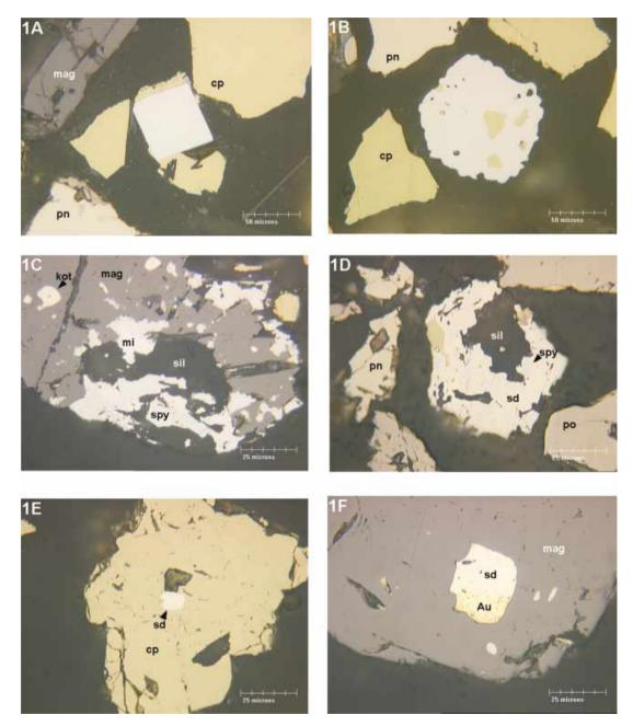
FIG. 1. Euhedral (1A) and anhedral (1B) grains of sperrylite (bluish white) in association with chalcopyrite (cp), pentlandite (pn), and magnetite (mag) C. Sperrylite (spy) and michenerite (mi) intergrown with a silicate mineral (sil) and magnetite (mag), which also contains an inclusion of kotulskite (kot). D–F. Sudburyite (sd) associated with sperrylite (spy), chalcopyrite (cp), magnetite (mag), and Au–Ag alloy (Au). Additional symbol: po: pyrrhotite.
