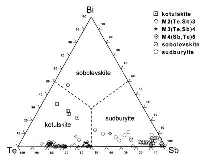
FIG. 3. Compositional variation of the sudburyite – kotulskite – sobolevskite solid solution in the Wellgreen deposit. Results of 43 analyses of sudburyite, kotulskite and sobolevskite and of 59 analyses of phases of the type  $Me(Te,Sb,Bi)_{1+x}$  are projected onto the Te–Bi–Sb ternary (atomic proportions).
