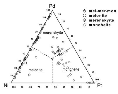
FIG. 7. Compositional variation of solid solution of palladoan melonite, merenskyite and moncheite in the Wellgreen deposit. Results of 93 analyses are projected onto the Ni – Pd – Pt ternary (atomic proportions). A grain with a composition representing <sup>1</sup>/<sub>3</sub> melonite, <sup>1</sup>/<sub>3</sub> merenskyite and <sup>1</sup>/<sub>3</sub> moncheite is shown as mel-mer-mon.
