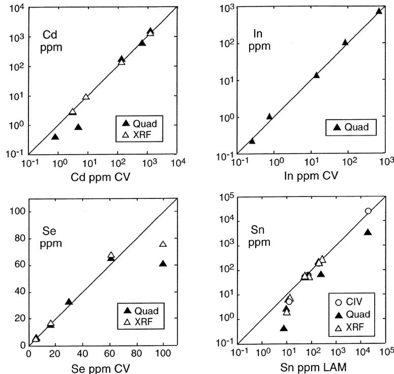
FIG. 8. A comparison of results for Cd, In, Se, and Sn obtained on the sulfide ore standards by solution ICP-MS analysis of whole-rock powders (filled triangles) with data obtained by LA-ICP-MS, XRF, and the reference values for these materials.
