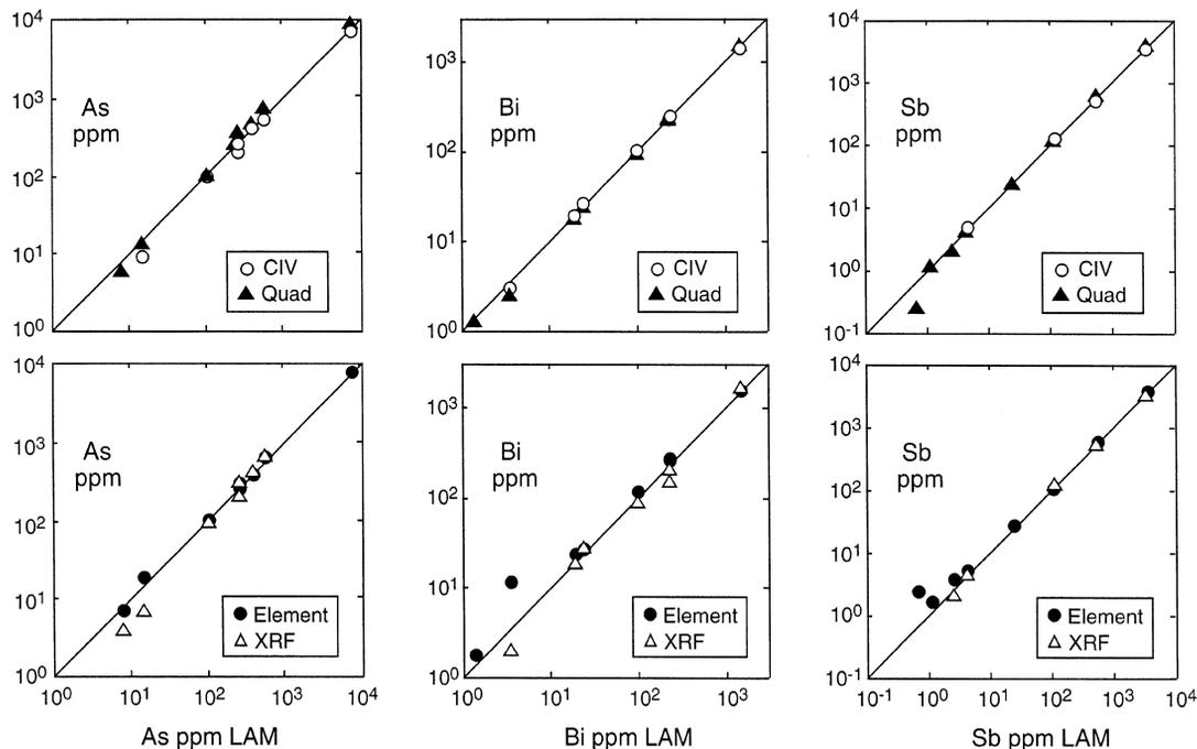
FIG. 7. A comparison of results for As, Bi, and Sb obtained on the fused sulfide ore standards by LA-ICP-MS with reference values for these materials (open circles), solution ICP-MS analysis of the fused glasses (filled circles), XRF (open triangles), and solution ICP-MS analysis of whole-rock powders (filled triangles).
