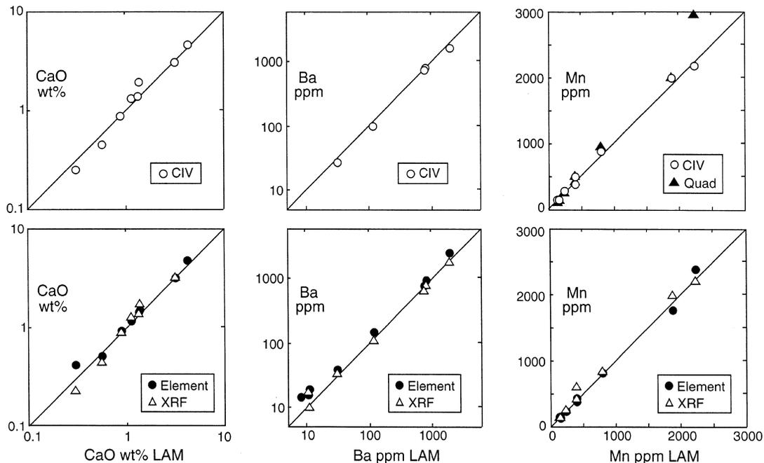
FIG. 4. A comparison of results for  $\text{CaO}$ ,  $\text{Ba}$ , and  $\text{Mn}$  obtained on the fused sulfide ore standards by LA-ICP-MS with reference values for these materials (CIV; open circles), solution ICP-MS analysis of the fused glasses (filled circles), XRF (open triangles), and solution ICP-MS of unfused whole-rock powders (filled triangles).
