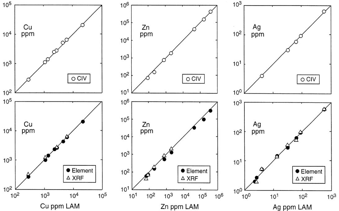
FIG. 5. A comparison of results for Cu, Zn, and Ag obtained on the fused sulfide ore standards by LA-ICP-MS with reference values for these materials (open circles), solution ICP-MS analysis of the fused glasses (filled circles), and XRF (open triangles).
