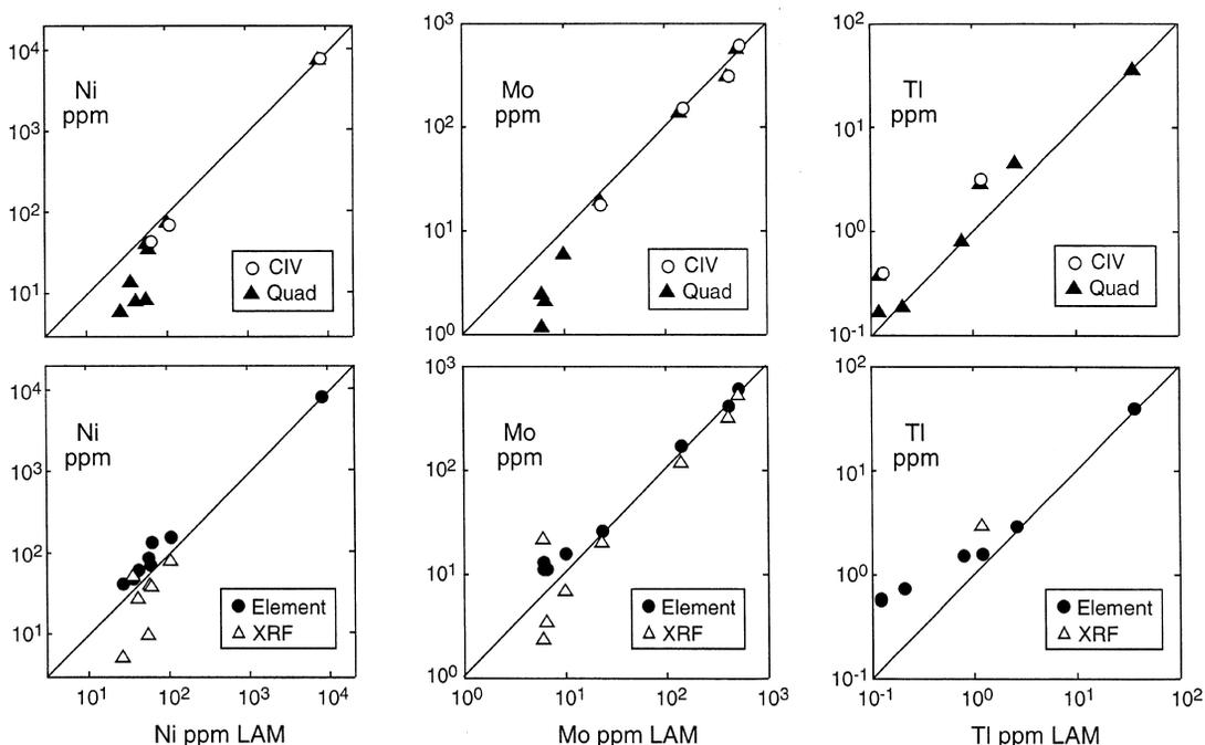
FIG. 9. A comparison of results for Ni, Mo, and Tl obtained on the sulfide ore standards by LA-ICP-MS with reference values for these materials (open circles), solution ICP-MS analysis of the fused glasses (filled circles), XRF (open triangles), and solution ICP-MS analysis of whole-rock powders (filled triangles).
