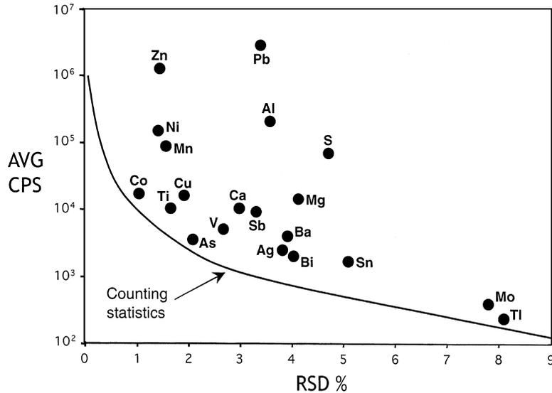
FIG. 2. Analytical precision, as indicated by the  $1\sigma$  RSD of replicate analyses of the calibration standard STDGL-1, exceeds that expected from counting statistics, indicating additional sources of analytical error.
