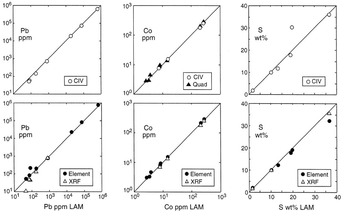
FIG. 6. A comparison of results for Pb, Co, and S obtained on the fused sulfide ore standards by LA-ICP-MS with reference values for these materials (open circles), solution ICP-MS analysis of the fused glasses (filled circles), XRF (open triangles), and solution ICP-MS analysis of whole-rock powders (filled triangles).
