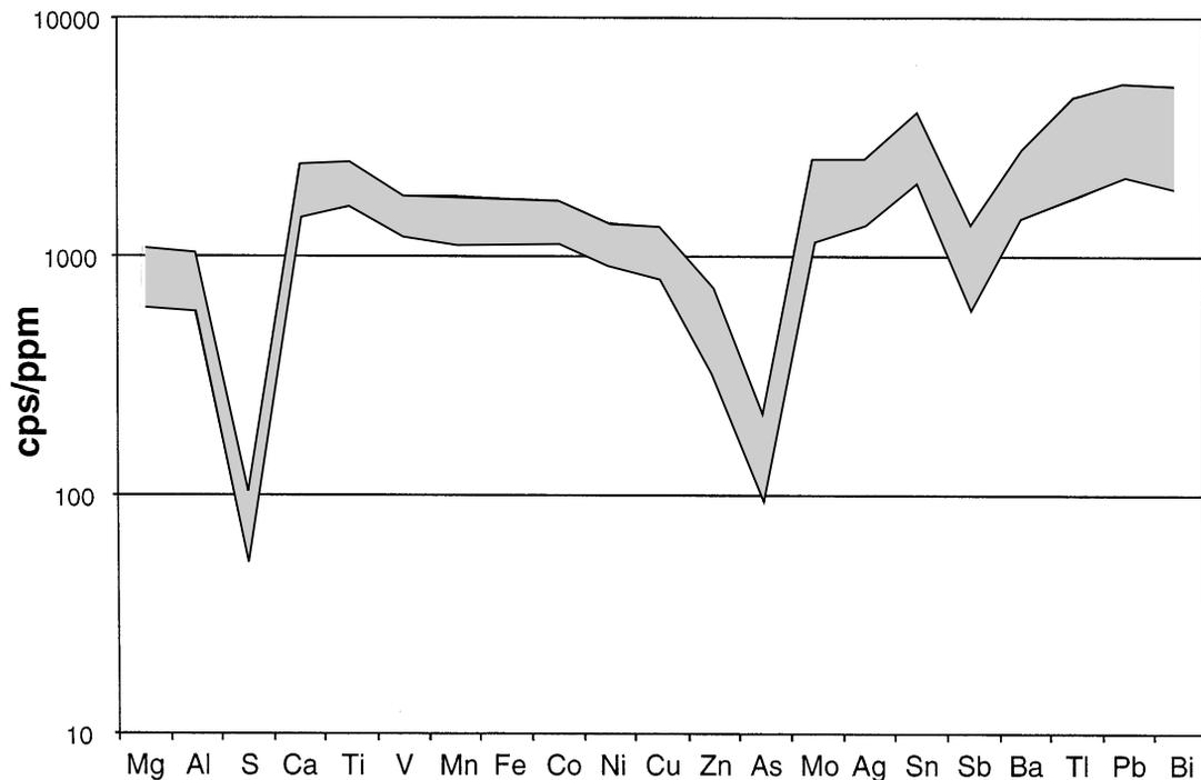
FIG. 1. Relative sensitivities (cps/ppm) of the elements determined on sulfide ores by laser-ablation ICP-MS analysis of fused glasses. Data are based on absolute abundances in the glass and have been normalized for isotopic abundance. The grey field represents the range encountered for the calibration standard STDGL-1 during this study.
