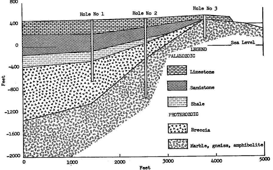
FIG. 5. A vertical section drawn through the three drill holes.
