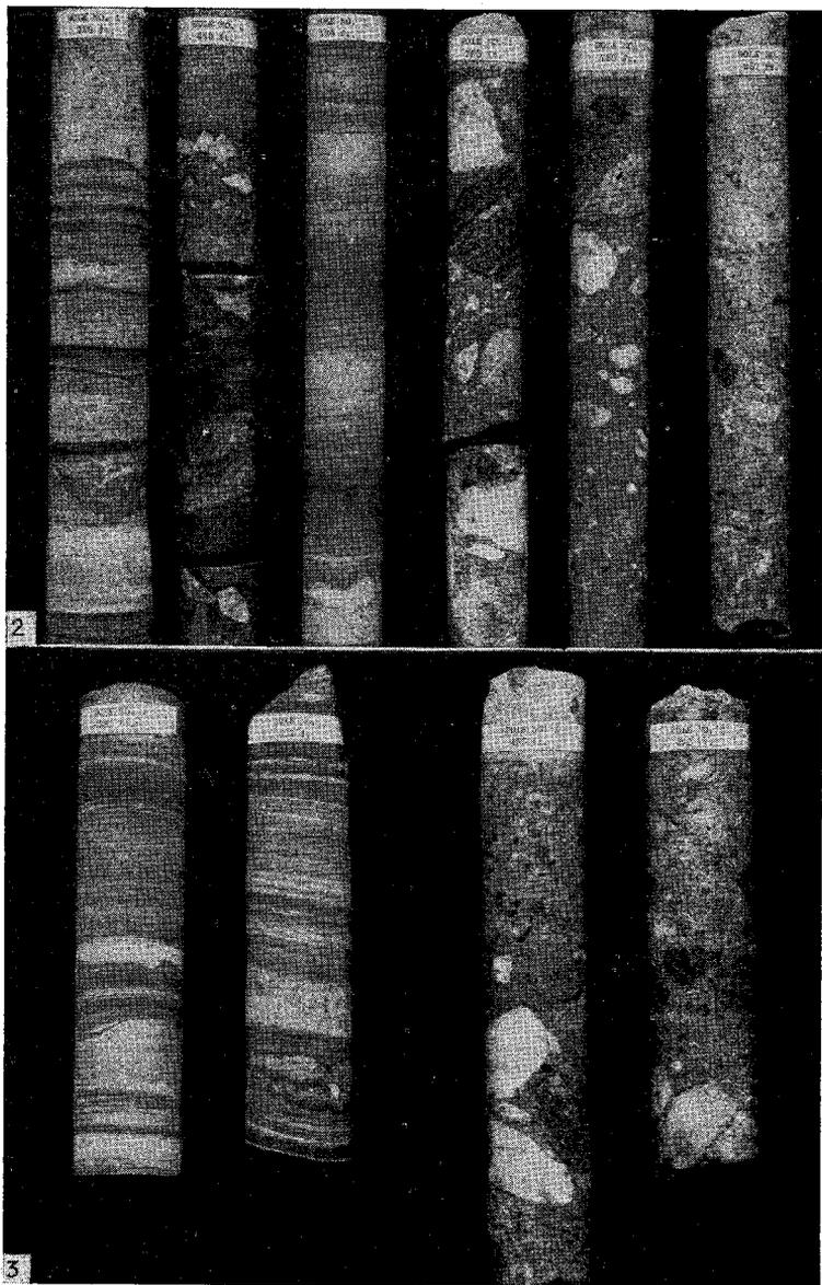
FIGS. 2 AND 3. Photographs of drill core from holes 1 and 2 showing from left to right the interbedded shale and sandstone and the underlying breccia.
