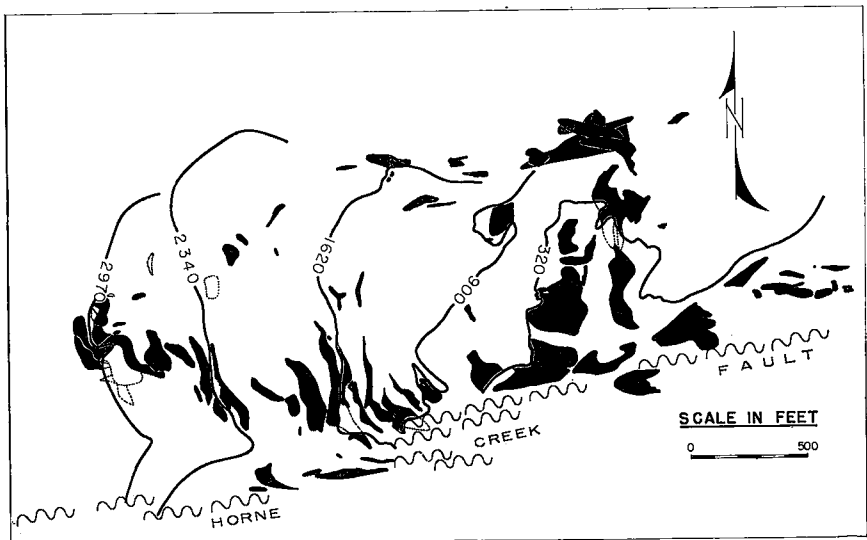
FIG. 3. Relationship of the ore (black) to the articular structure and the Horne Creek fault. Contours show footwall of porphyritic rhyolite.
