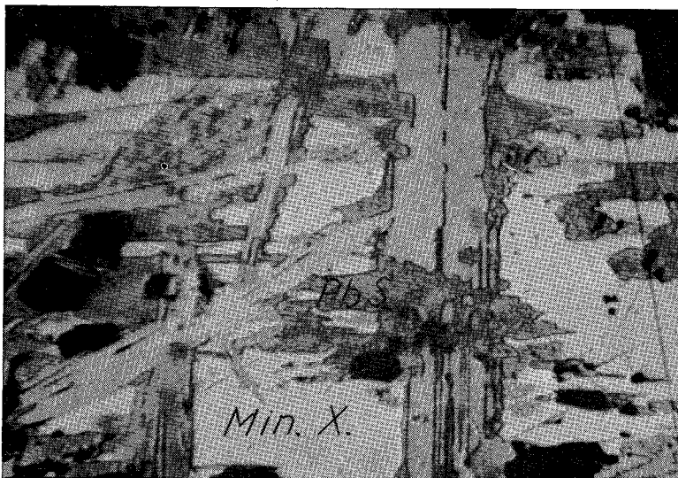
FIG. 6. Polished section. 180X. Nicols crossed at 25°. Etched 1-2 secs, with conc. HNO 3 .
