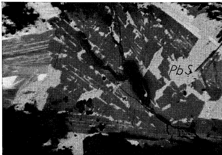
FIG. 1. Polished section, 140X. Nicols crossed at 88°.
