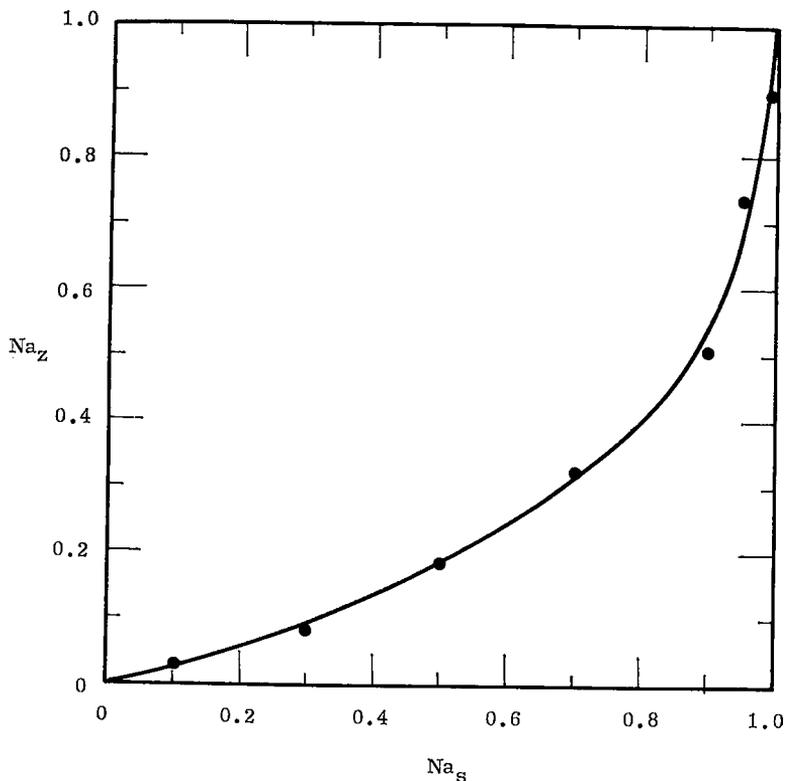
FIG. 2. The 23 °C isotherm for the reaction  $K_z + Na_s \rightleftharpoons Na_z + K_s$  with stilbite. Total equilibrium solution normality was constant at 1.0.
