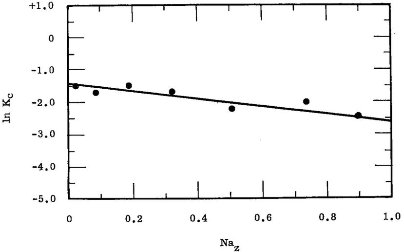
FIG. 6. A graph of the corrected selectivity quotient,  $K_s$ , versus the equivalent fraction of sodium on the zeolite,  $Na_z$ , for the reaction  $K_z + Na_s \rightleftharpoons Na_z + K_s$  at 23 °C with stilbite.
