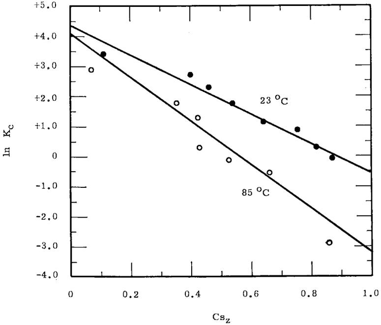
FIG. 5. A graph of the corrected selectivity quotient,  $K_s$ , versus the equivalent fraction of cesium on the zeolite, at 23 °C and 85 °C for the reaction  $Na_z + Cs_s \rightleftharpoons Cs_z + Na_s$  with stilbite.
