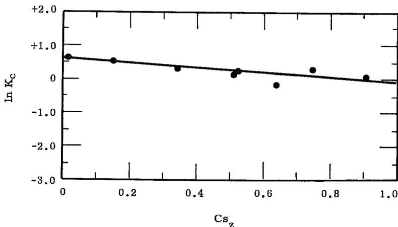
Fig. 7. A graph of the corrected selectivity quotient,  $K_c$ , versus the equivalent fraction of cesium on the zeolite,  $Cs_2$ , for the reaction  $K_z + Cs_2 \rightleftharpoons Cs_{2z} + K_z$  at 23 °C with stilbite.
