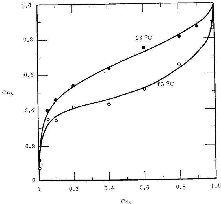
FIG. 1. The 23 °C and 85 °C isotherms for the reaction  $Na_z + Cs_s \rightleftharpoons Cs_z + Na_s$  with stilbite. Total equilibrium solution normality was constant at 1.0.  $Cs_z$  = equivalent fraction of cesium on the zeolite.  $Cs_s$  = equivalent fraction of cesium in the equilibrium solution.
