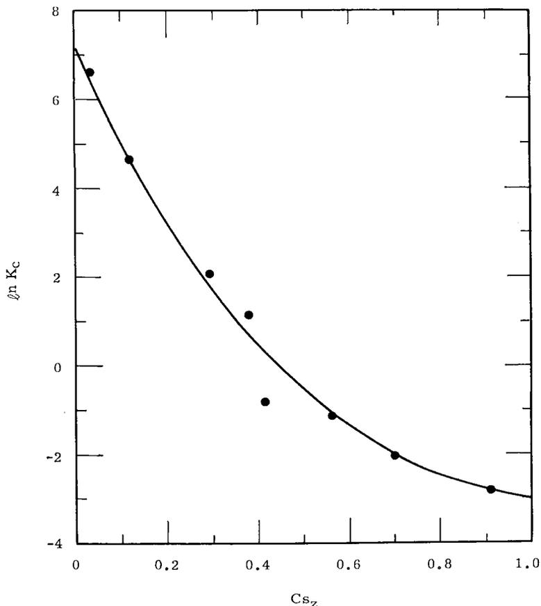
FIG. 8. A graph of the corrected selectivity quotient,  $K_c$ , versus the equivalent fraction of cesium on the zeolite,  $Cs_Z$ , for the reaction  $Sr_Z + 2Cs_Z \rightleftharpoons 2Cs_Z + Sr_Z$  at 23 °C with stilbite.
