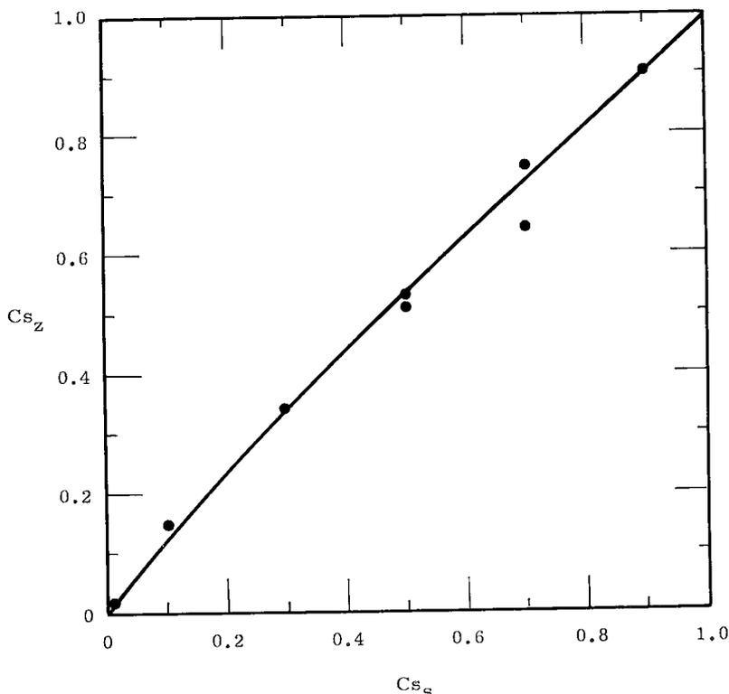
FIG. 3. The 23 °C isotherm for the reaction  $K_z + Cs_s \rightleftharpoons Cs_z + K_s$  with stilbite. Total equilibrium solution normality was constant at 1.0.
