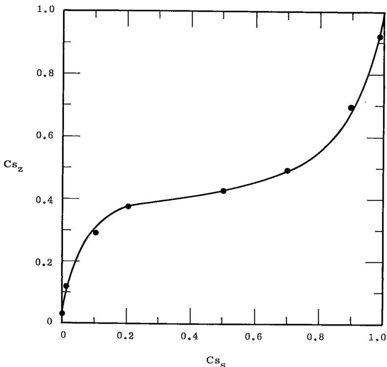
FIG. 4. The 23 °C isotherm for the reaction  $Sr_z + 2Cs_s \rightleftharpoons 2Cs_z + Sr_s$  with stilbite. Total equilibrium solution normality was constant at 1.0.  $Cs_z$  = equivalent fraction of cesium on the zeolite.  $Cs_s$  = equivalent fraction of cesium in the equilibrium solution.
