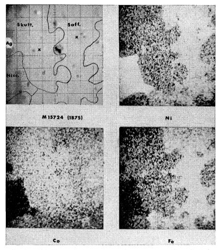
FIG. 2. Top left. Electron backscatter image of intergrown skutterudite and safflorite. Other photographs are x-ray scanning images of  $K\alpha_1$  radiations. The area covered by these scans is the same as that of the electron backscatter. Note the relative preferential inclusion of Ni and Fe in safflorite, and Co in skutterudite. Sample from Mississagi, Ontario (ROM, M15724). Grid scale = 0.03 mm.
