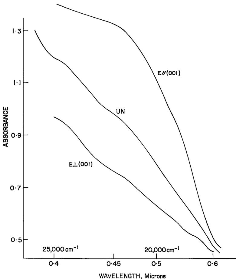
FIG. 5. Absorption spectrum of clintonite section cut  $\perp(001)$   $l = \sim 0.03$  cm.
