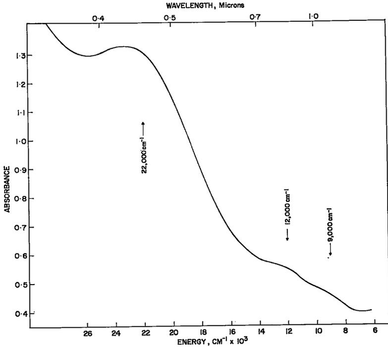
FIG. 4. Absorption spectrum of 001 section of clintonite in unpolarized light.  $l = 0.05$  cm.
