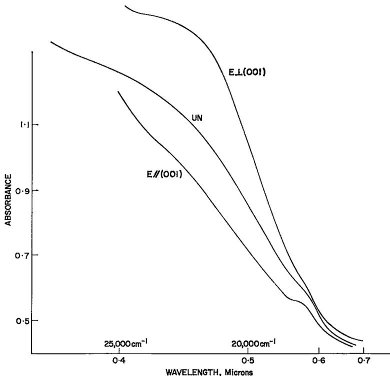
FIG. 3. Absorption spectrum of section of astrophyllite cut  $\perp$ (001).  $l = \sim 0.03$  mm.
