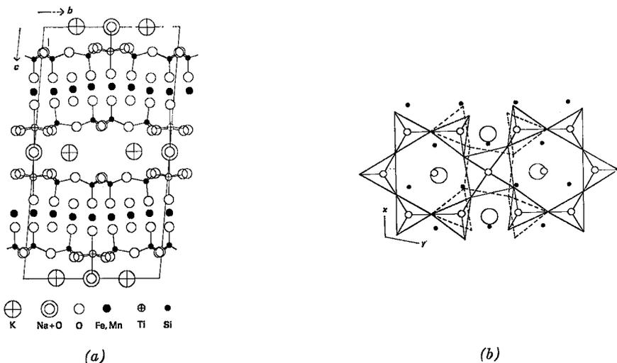
FIG. 1. Crystal structure of astrophyllite after Woodrow (1967). (a) is projection along the  $x$  axis. (b) is projection along  $[001]$  of one layer ( $z = 0$  to  $z = c/4$ ) of the structure. Black dots = Fe atoms at approximately  $z = c/4$ ; large circles = alkali ions at  $x = 0$ ; small circles = oxygen atoms. Dashed lines indicate an alternative arrangement.
