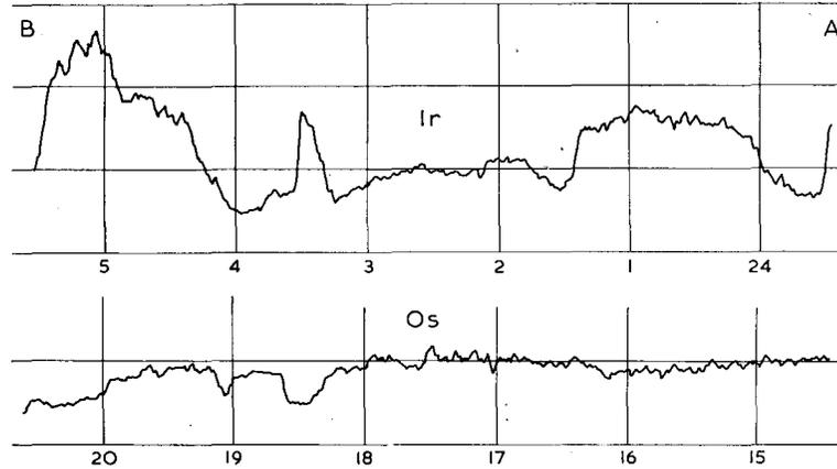
FIG. 6. The variation in Ir and Os concentrations within a single grain of  $\text{Pt}(\text{Ir},\text{Os})_2\text{As}_4$ ; the traverse is from A to B in the grain marked in pl. XVII, fig. 2.
