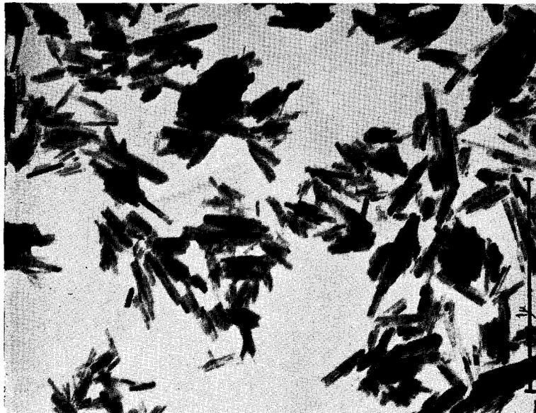
FIG. 1. Electron micrograph of crystals of akaganéite.
