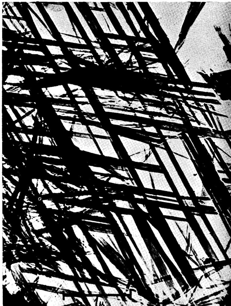
FIG. 2. Electron micrograph of a mat showing two texture axes for the  $\beta$ -FeOOH crystals composing it, which had transformed in the solid from  $\text{FeCl}_2 \cdot 4\text{H}_2\text{O}$ .
