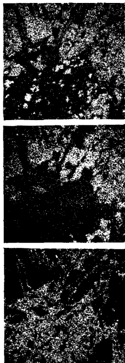
FIG. 1. X-ray scanning photographs of an area on the calciotantalite specimen containing mainly intergrown microlite and tin-rich tantalite. A few small areas of 'normal' tantalite are visible; these contain iron but no tin. Top, Fe- K\alpha ; middle, Sn- L\alpha ; bottom, Ca- K\alpha . \times 40 .
