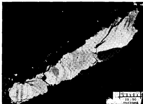
FIG. 3. Parkerite vein (lower left-hand in fig. 1) showing details of parkerite twinning and largest grain of niggliite (dark grey). A few degrees from extinction.
