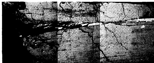
FIG. 1. BSE photograph showing wodgeinite (medium grey) cut by a vein of tapiolite (white) and cassiterite/'staringite' (dark grey); the length of the scale bar is 1 mm.
