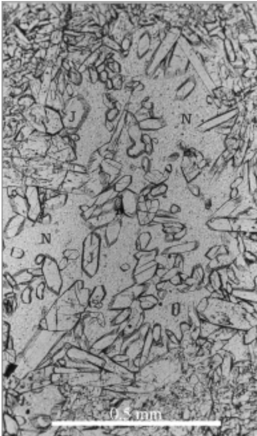
FIG. 4. Euhedral crystals of jadeite in natrolite (PPL). J = jadeite, N = natrolite.
