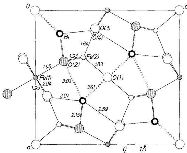
Fig. 5. Schematic representation of the structure of  $\text{Bi}_2\text{Fe}_4\text{O}_9$ . Explanations for symbols and figures are same as in Fig. 2
