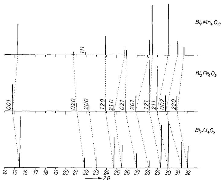
Fig. 1. Graphical representation of x-ray powder-diffraction patterns of  $\text{Bi}_2\text{Mn}_4\text{O}_{10}$ ,  $\text{Bi}_2\text{Al}_4\text{O}_9$ , and  $\text{Bi}_2\text{Fe}_4\text{O}_9$ . Patterns were obtained by diffractometer with  $\text{CuK}\alpha$  radiation
