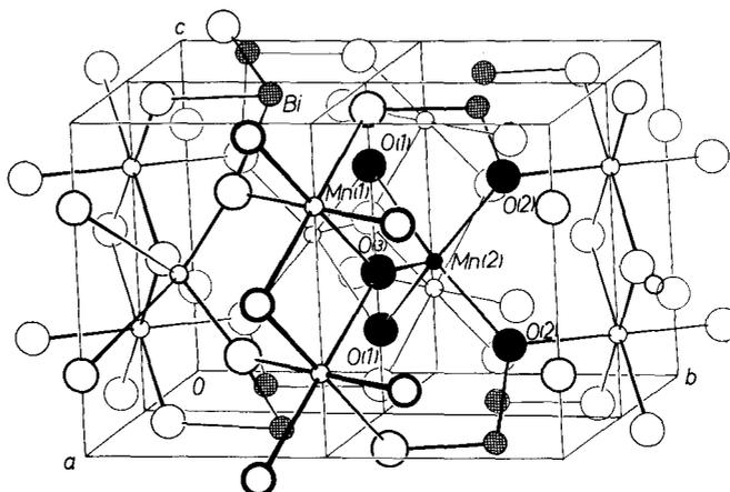
Fig. 6. Structural scheme of  $\text{Bi}_2\text{Mn}_4\text{O}_{10}$ . Large circles represent oxygen, small circles manganese, and cross-hatched circles bismuth atoms. A square-pyramidal coordination is indicated by black coloring of related atoms
