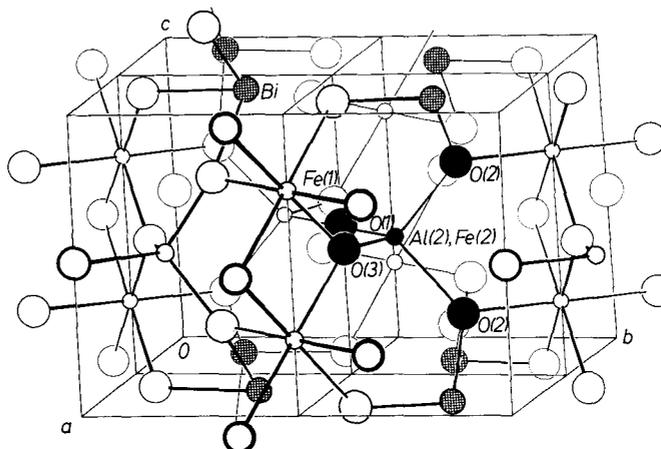
Fig. 7. Structural scheme of  $\text{Bi}_2\text{Al}_4\text{O}_9$ , and  $\text{Bi}_2\text{Fe}_4\text{O}_9$ . Large circles represent oxygen, small circles aluminum or iron, and cross-hatched circles bismuth atoms. A tetrahedral coordination is indicated by black coloring of related atoms
