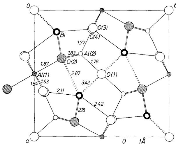
Fig. 4. Schematic representation of the structure of  $\text{Bi}_2\text{Al}_4\text{O}_9$ . Explanations for symbols and figures are same as in Fig. 2
