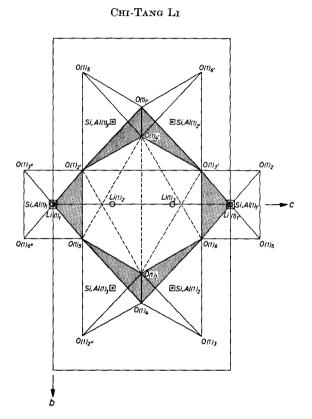
Fig. 2. The projection of LiAlSi<sub>2</sub>O<sub>6</sub> III on (100)
