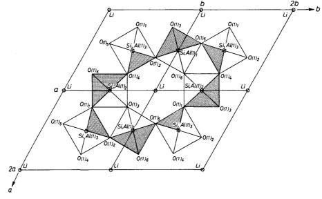
Fig. 1. The projection of LiAlSi<sub>2</sub>O<sub>6</sub> III on (001)
