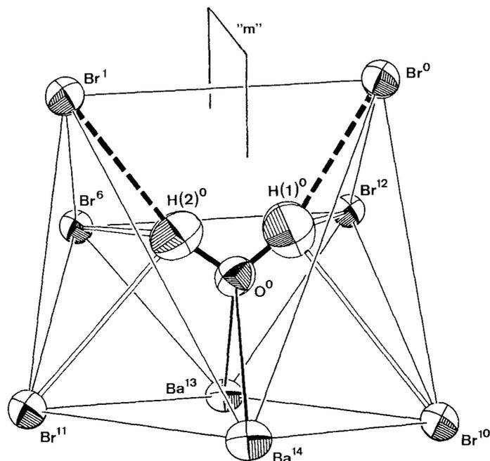
Fig. 3. Environment of the water molecule in  $\text{BaBr}_2 \cdot 2\text{H}_2\text{O}$ . Dashed lines represent the shortest hydrogen bonds, longer  $\text{H}\cdots\text{Br}$  distances are designated by open lines. The pseudo mirror plane is indicated by "m". See Table 3 for symmetry operations.
