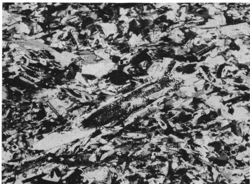
Fig. 3. — Elongated prism of hornblende showing ilmenitic exsolutions and a «hollow shell crystal» structure. (crossed Nicols 60 \times ).
