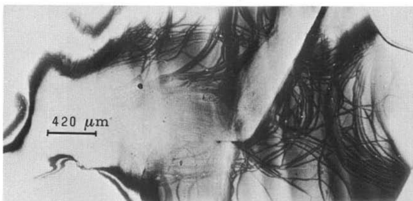
Fig. 7. — X-ray traverse-topograph: (reflexion (11\bar{2}0) ). Evidence is seen of the large production of basal dislocation and of their movement due to the low stresses that occurred during the handling of the specimen (compare with figure 6).
