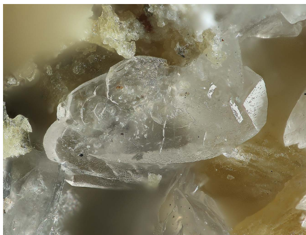
FIGURE 1. Lenticular crystals of smamite from Giftgrube mine, Sainte-Marie-Aux-Mines. Horizontal field of view is 0.6 mm (photo W. Perraud). (Color online.)
