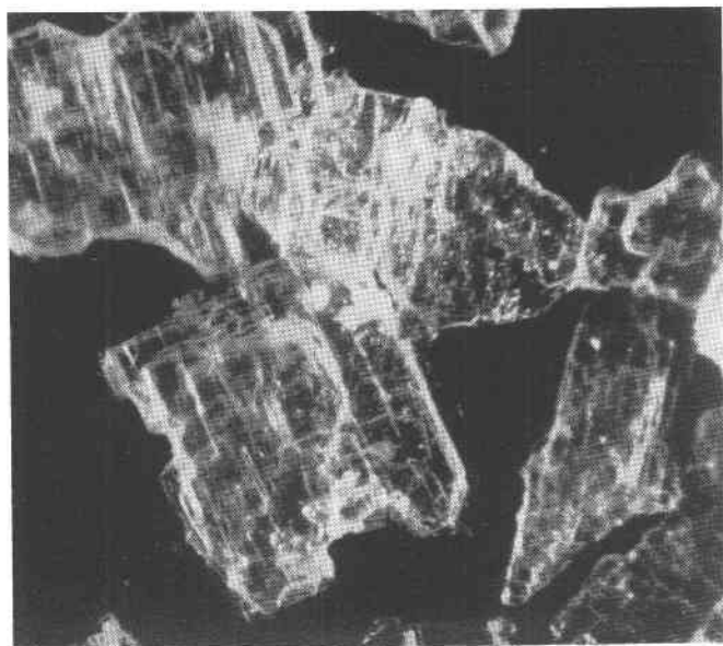
FIG. 3. Cleavage fragments of metaheinrichite from Oregon lying on (001), showing traces of (100) and (010) cleavages. \times 100 .
