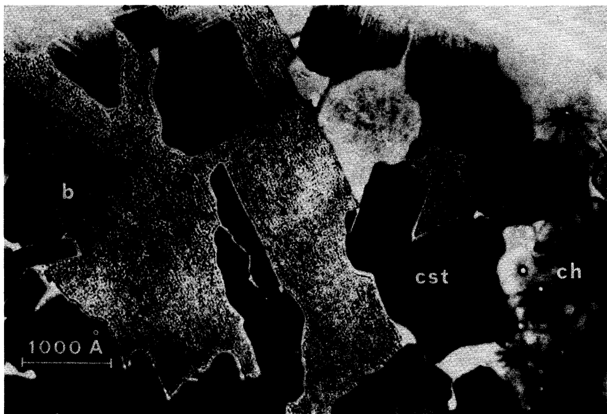
Fig. 3. TEM image showing association of fibrous carlosturanite (cst), brucite (b) and chrysotile (ch) as seen along the fiber axis.
