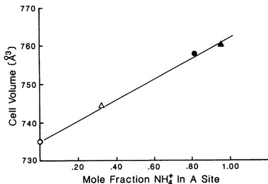
Fig. 2. Unit-cell volume (Table 1) vs. mole fraction  $\text{NH}_4^+$  in the A site of ammonioalunite. Dots represent synthetic samples, open is from Menchetti and Sabelli (1976) and solid is from this study. Triangles represent natural samples discussed in this study, open is from the Ivanhoe mine, Nevada, and solid is from The Geysers, California.
