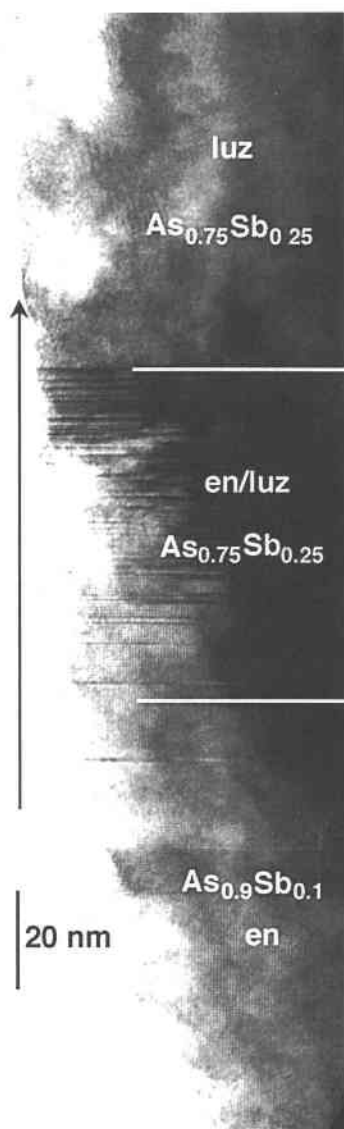
FIGURE 3. Intergrowth of enargite and luzonite. The atoms per formula unit are shown for As and Sb for both phases. A structurally disordered zone is marked "en/luz." The arrow shows the assumed direction of crystal growth (see Discussion).
