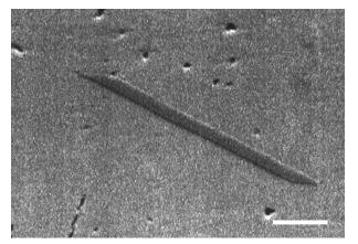
**FIGURE 1.** Allabogdanite crystal in plessite matrix. Etched. Secondary electron image. Scale bar 10 μm.
