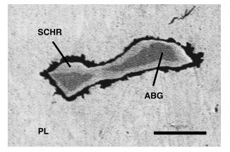
FIGURE 3. Relict of allabogdanite crystal (ABG) surrounded by schreibersite rim (SCHR) in plessite matrix (PL). Black phase is a secondary Fe-Ni-hydroxide. Backscattered electron image. Scale bar 10 µm. morph of (Fe,Ni)<sub>2</sub>P, by analogy with iron manganese phosphide, FeMnP, studied by Chenevier et al. (1987).
